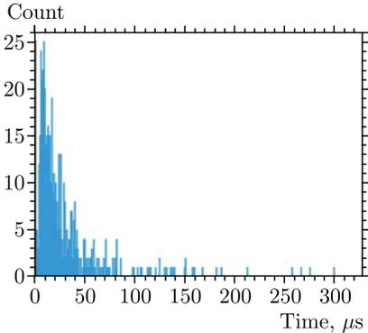
Fig. 5. Distribution of time differences between neutron detection and the spontaneous fission of  $^{246}\text{Fm}$
