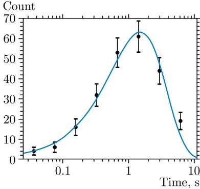
Fig. 3. Distribution of time differences between recoil nuclei and fission fragments registration for  $^{246}\text{Fm}$  (dots) and fitting by method [11] (curve)
