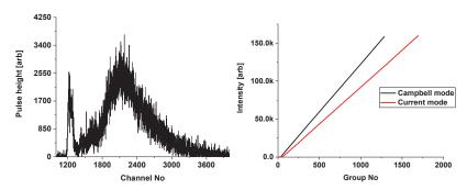
Figure 8. On the left; group waveform composed of 100 sequential waveforms; on the right comparison of intensity measurement in Campbell and current modes demonstrates very good linearity.
