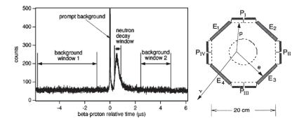
**Fig.3.** Spectrum of double electron-proton coincidences obtained by emiT Group [11] with two peaks and ion background value comparable to the neutron decay peak; emiT group scheme for registering beta electron and recoil proton.
