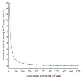
Fig. 4. Saturation specific activity of <sup>24</sup>Na as a function of ion-exchange removal rate in primary coolant of AP-1000
