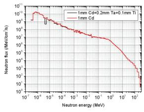
Figure 3. Neutron spectrum of CSNS back-n
