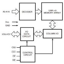
Fig. 1. Functional schematic of IS62WV1288DBLL.
