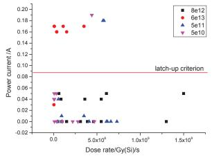
Fig.1 Transient ionizing latch-up effect of neutron irradiated IDT6116 SRAMs.
