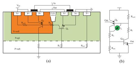
Fig.3 The parasitic P-N-P-N structure in CMOS devices and the equivalent circuitry:
