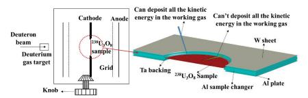
**Fig. 1.** The sketch of the experimental setup.
