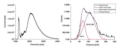
Figure 7. On the left: FC pulses summed for 160000 reactor bursts. On the right: radiation from the reactor burst with decomposition into the neutron (partially moderated/resonance) and gamma plus fast neutrons, escaped the moderator, represented by Gaussians. S indicates relative area under the Gaussians.
