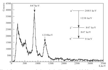
Fig. 4. Gamma-spectrum for iron, obtained by "Romasha" BGO γ-detector system.
