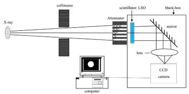
**Fig.1** CCD camera imaging energy spectrum measuring system for pulsed gamma/X. Gamma/X rays are collimated to parallel beams, and irradiated directly onto the 16 holes of attenuators and the rear scintillator (e.g. LSO). The emission light is reflected by a mirror to the lens of CCD camera. The CCD signal is transferred to computer and can be displayed through developed software. The grey levels represent the intensity of incident gamma/X measured.
