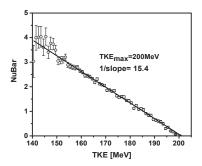
**Fig. 6.** The average PFN emission distribution mass dependence, measured in <sup>235</sup>U(n<sub>th</sub>,f)reaction in comparison with data from Ref. [7].
