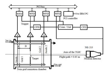
**Fig. 1.** Experimental Setup.
