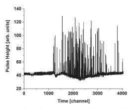
Figure 2. Recorded waveform of single burst of the IBR2M (full range is 20500 us).
