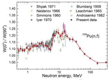
Fig. 6. Anisotropy of fission fragments of <sup>239</sup>Pu.
