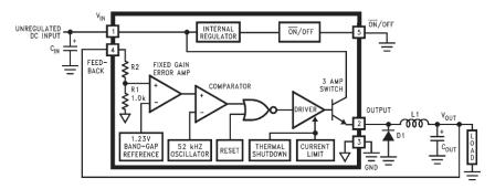
Fig. 2. Functional schematic of LM2576T-3.3.
