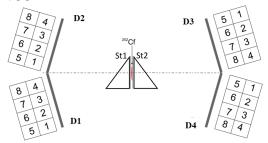
**FIGURE 1.** Ex1: layout of the experimental setup. The <sup>252</sup>Cf (sf) source is placed between two "start" micro-channel plates based timing detectors *St1* and *St2*. Four mosaics (D1÷D4) of eight PIN diodes each provide measuring of both the FF energy and time-of-flight.
