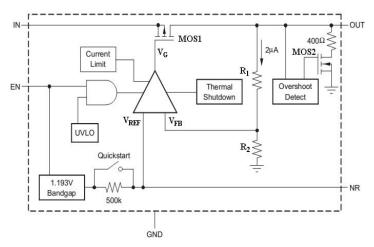
Fig. 7. Functional block diagram of the device.
