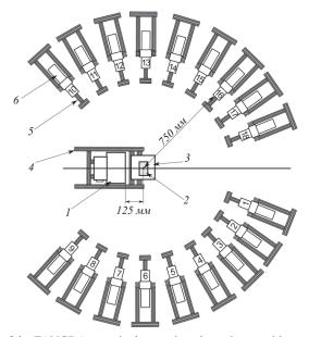
Fig. 1. Scheme of the TANGRA setup in the reaction plane: I – portable neutron generator ING-27, 2 – sample at the center of "Romasha"  $\gamma$ -ray registration system, 3 – sample holder, 4 – generator support, 5 –  $\gamma$ -ray detector holder, 6 – BGO  $\gamma$ -ray detector. The "tagged" neutron beam direction is indicated by horizontal plain line.
