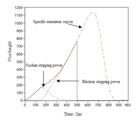
FIG.6. The specific energy losses of primary fission products obtained by the Frisch-grid ionization chamber.
