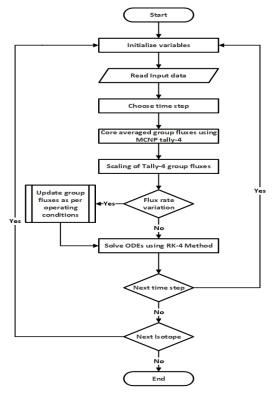
Fig. 3. Flowchart of CPA-AP100 for computing CPA under steady-state operation and flux rate vitiation
