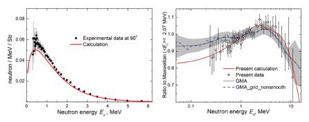
**Fig. 4.** Left – the PFN spectrum measured for angle 90° relative to the fission fragment direction. Right – the total PFN spectrum of  $^{239}$ Pu(n,f) obtained by summing over angles  $\theta$  are shown as a ratio to Maxwell distribution. GMA – generalized least square fit of PFN spectra measured by different experimental groups (non-model evaluation) – taken from ref. [10].
