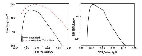
**Fig. 11.** Comparison of measured PFN velocity distribution with Maxwell distribution in <sup>252</sup>Cf(sf) experiment.
