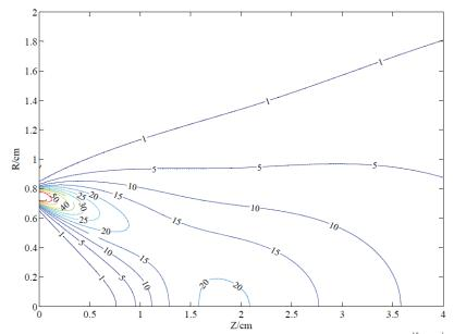
Fig. 2. The contour line of the gas density (the unit for the number density is 10<sup>16</sup> cm<sup>-3</sup>).
