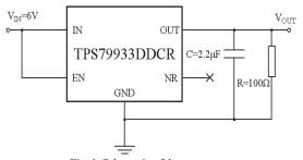
Fig. 1. Schematic of the test system.
