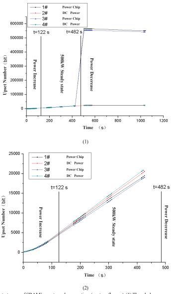
Fig. 5. The test curve of SRAM's upset number over time (neutron fluence). (1) The whole process of reactor's operation. (2) Operation of reactor's steady state.
