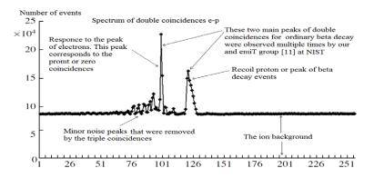
**Fig.2.** Timing spectrum for e-p coincidences. Each channel corresponds to 25 ns. The peak at channel 99–100 corresponds to the prompt (or zero) coincidences. The coincidences between the decay electrons and delayed recoil protons (e-p coincidences) are contained in the large peak centered at channel 120.
