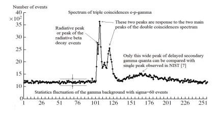
**Fig.6.** Timing spectrum for triple e-p-g coincidences. Each channel corresponds to 25 ns. In this spectrum, three main peaks in channels 103, 106 and 120 can be distinguished. The leftmost peak in 103 channel among these three main peaks is connected with the peak of radiative decay events.
