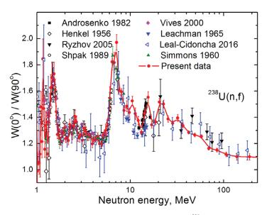
Fig. 4. Anisotropy of fission fragments of <sup>238</sup>U.
