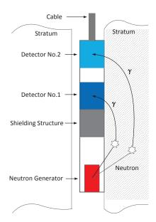
Fig. 1. The structure of D-G well logging instrument.
