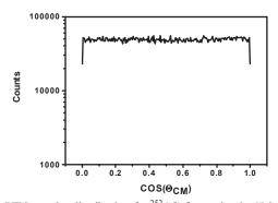
Fig. 10. PFN angular distribution for <sup>252</sup>Cf(sf) reaction in CM reference frame.
