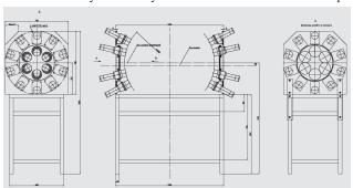
Fig. 17. Fast neutron detector composed of 32 liquid scintillation modules with position sensitive twin ionization chamber in centre (not shown in figure)
