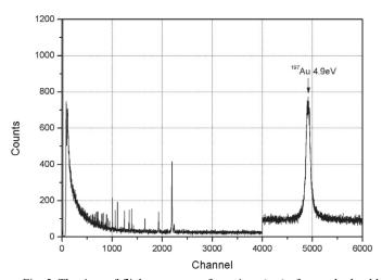
Fig. 5. The time-of-flight spectrum of reactions  $(n,\gamma)$  of a standard gold sample.
