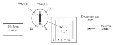
1- Cathode; 2- Grid; 3- Anode; 4- Shield
