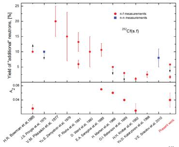
**Fig. 1.** Main results of previous investigations of PFN emission mechanism for <sup>252</sup>Cf: upper part - yield of "scission" neutrons (downward and upward arrows indicate the upper and lower bounds, respectively); lower part - anisotropy of the angle distribution of PFNs in the center-of-mass system of fission fragments.
