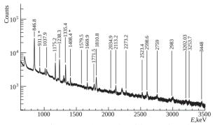
Fig. 3. Gamma-spectrum for Fe (HPGe). Energies of the most intensive  $\gamma$ -transitions  $E_{\gamma}$  (in keV) from reactions  $^{56}$ Fe(n,n'),( n,2n') are signed. Lines generated by reaction (n,2n') are marked with an asterisk.
