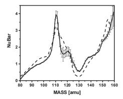
Fig. 7. The average PFN emission distribution dependence on FF TKE, measured in  $^{235}U(n_{th},f)$  reaction with  $Q_{max}{=}\sim\!205$  MeV.
