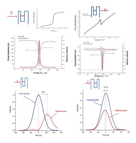
**Fig.2.** Above: reflection coefficient and the GDT for three-layer structures differing in the order of the layers. Below: relative magnitude and time relations between short wave packets incident and reflected from the same structures.
