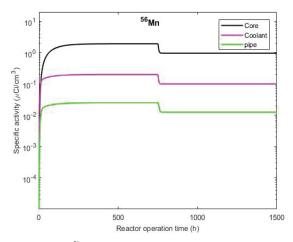
Fig. 9. The specific activity of <sup>56</sup>Mn in primary coolant and on inner walls of the primary system during normal operation and design-based variation in neutron flux rate
