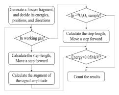
Fig. 3. The flowchart of the Mote Carlo simulation.
