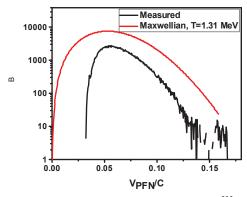
**Fig. 8.** Comparison of PFN velocity distribution, measured in <sup>235</sup>U(n<sub>th</sub>,f) reaction with Maxwell distribution with temperature parameter kT=1.31 MeV.
