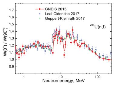
Fig. 8. Anisotropy of fission fragments of <sup>235</sup>U.
