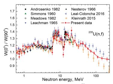
Fig. 3. Anisotropy of fission fragments of <sup>235</sup>U.
