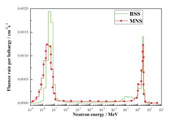
Fig. 4 Background neutron spectrum of laboratory
