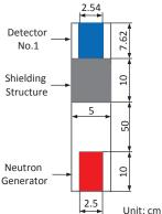
Fig. 2. The simulating model of the well logging instrument.
