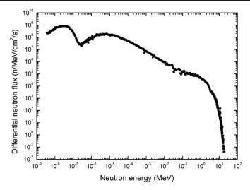
Fig. 2. Differential neutron flux at XAPR.
