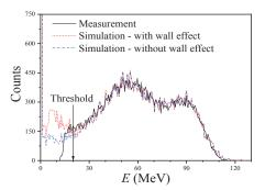
**Fig. 6.** The energy spectra of the neutron induced fission fragments. The solid line is the measured one. The dashed line and the dash dotted line are the simulated ones with and without considering the wall effect, respectively.
