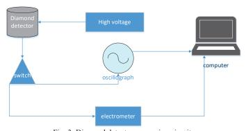
Fig. 3. Diamond detector measuring circuit.
