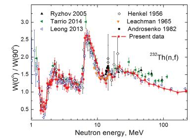
Fig. 5. Anisotropy of fission fragments of <sup>232</sup>Th.
