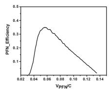
Fig. 9. PFN detection efficiency dependence on velocity measured in speed of light (C) units.
