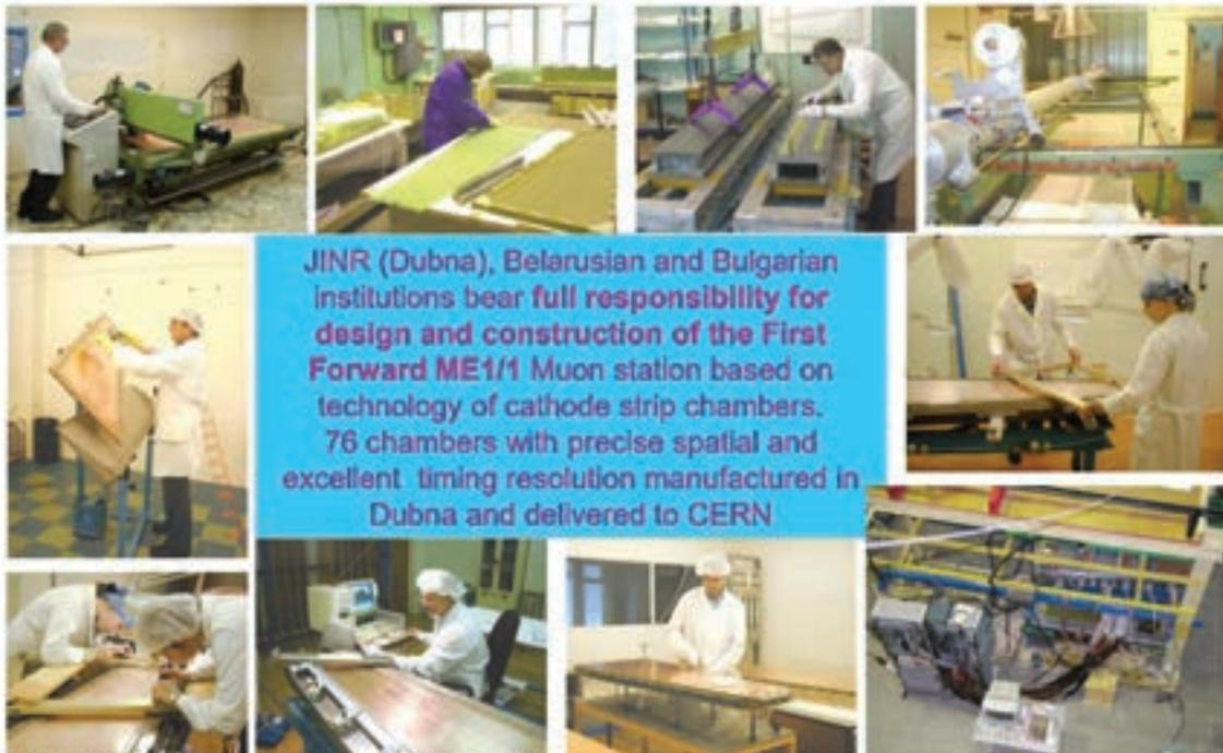
JINR (Dubna), Belarusian and Bulgarian institutions bear full responsibility for design and construction of the First Forward ME1/1 Muon station based on technology of cathode strip chambers. 76 chambers with precise spatial and excellent timing resolution manufactured in Dubna and delivered to CERN
