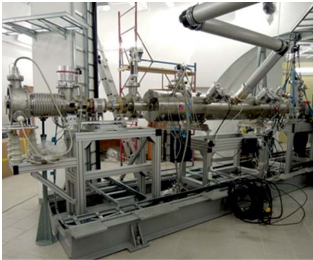
Initial part of the heavy ion linear accelerator of the NICA collider complex
