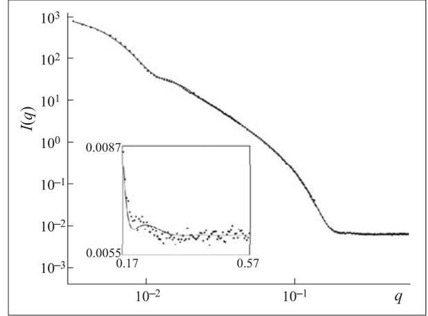
Fig. 5. The results of fitting the experimental data obtained at the small-angle spectrometer SANS-I, PSI (Switzerland)
