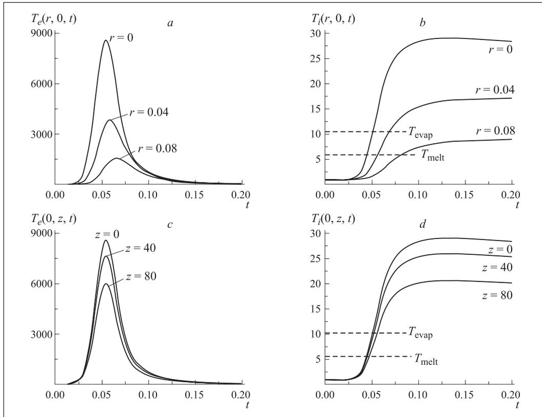
Fig. 6. Time dependence of the temperature of electron gas (a) and lattice (b) on the surface ( $z = 0$ ) of nickel irradiated with uranium ions for various distances from the track axis. Time dependences of temperatures of electron gas (c) and lattices (d) in the place of passing a uranium ion through a surface ( $r = 0$ ) for different depths  $z$  in the target. The shaded straight lines on panels b and d show the temperatures of melting  $T_{\text{melt}}$  and evaporation  $T_{\text{evap}}$
