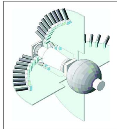
Fig. 3. The upgraded LNS setup at the internal beam of the Nuclotron. The scintillation detectors (36) mounted in four planes are directed towards the internal target area (spherical area)
