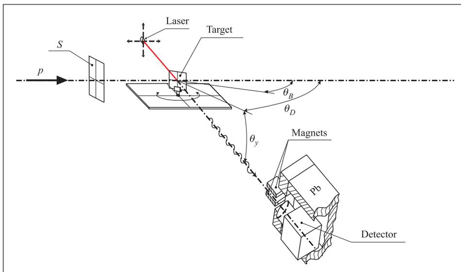
Fig. 10. Schematic diagram of the experimental setup:  $S$  is the ionization monitor of the beam,  $\theta_B$  is the crystal orientation angle, and  $\theta_D$  and  $\theta_y$  are the detection angles
