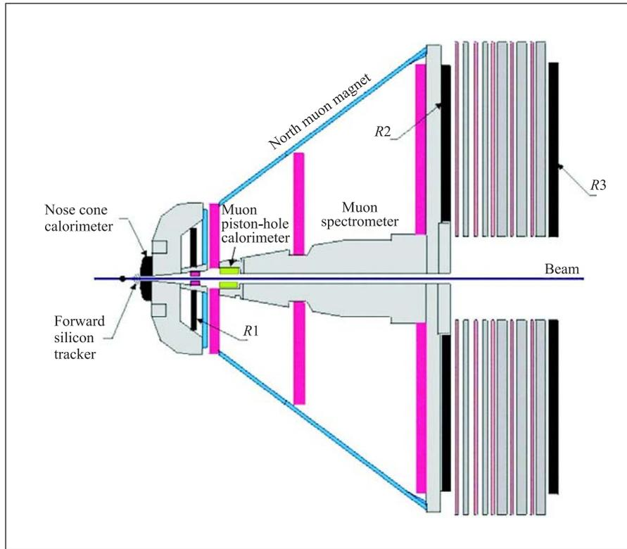
Fig. 18. Layout of the nose cone calorimeter for PHENIX. The calorimeter consists of tungsten plates and semiconductor detectors
