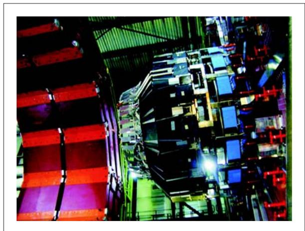
Fig. 20. The view of the hadron endcap calorimeter with the installed readout system for CMS
