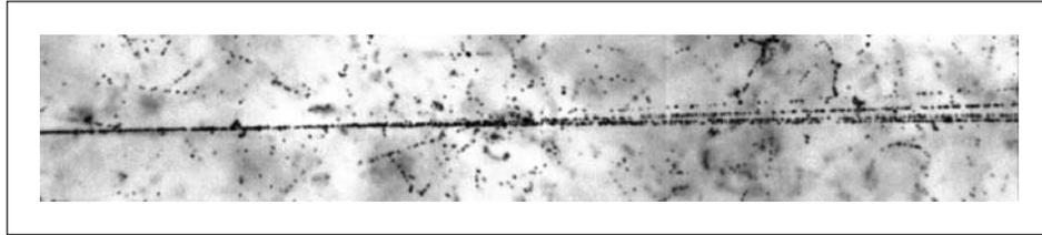
Fig. 9. Reconstructed image of dissociation of the  $2.1 A \cdot \text{GeV}$   ${}^{14}\text{N}$  nucleus in emulsion into one H and three He nuclei without production of target nuclear fragments and mesons («white» star)
