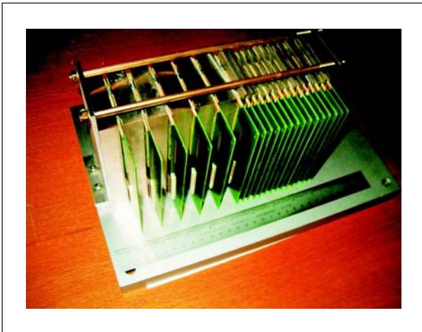
Fig. 19. Prototype of the nose cone Calorimeter for PHENIX
