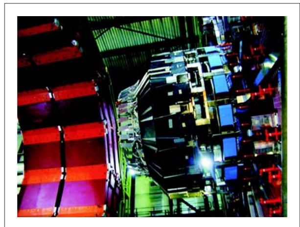
Fig. 20. The view of the hadron endcup calorimeter with the installed readout system for CMS
