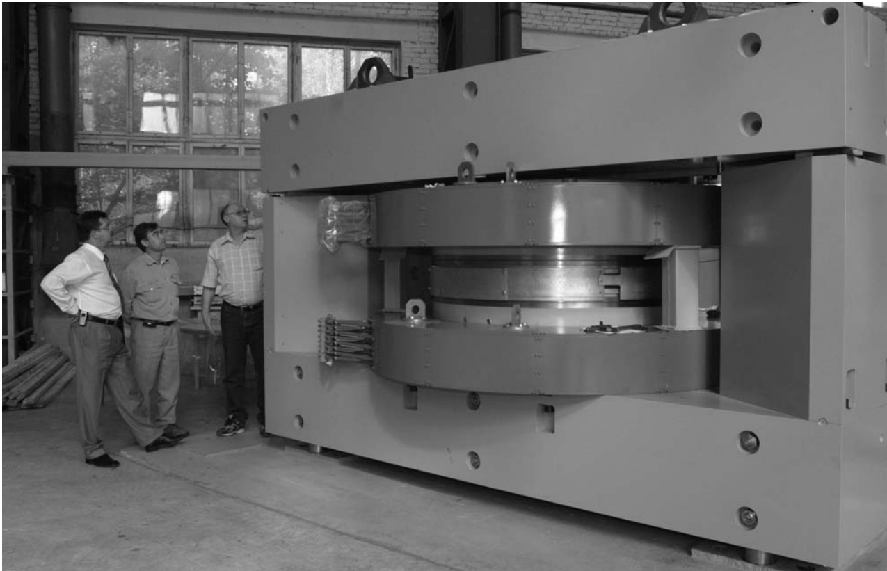
Dzhelepov Laboratory of Nuclear Problems, building 5. DC60 cyclotron, worked out at FLNR for Kazakhstan, at the final stage of assembling
