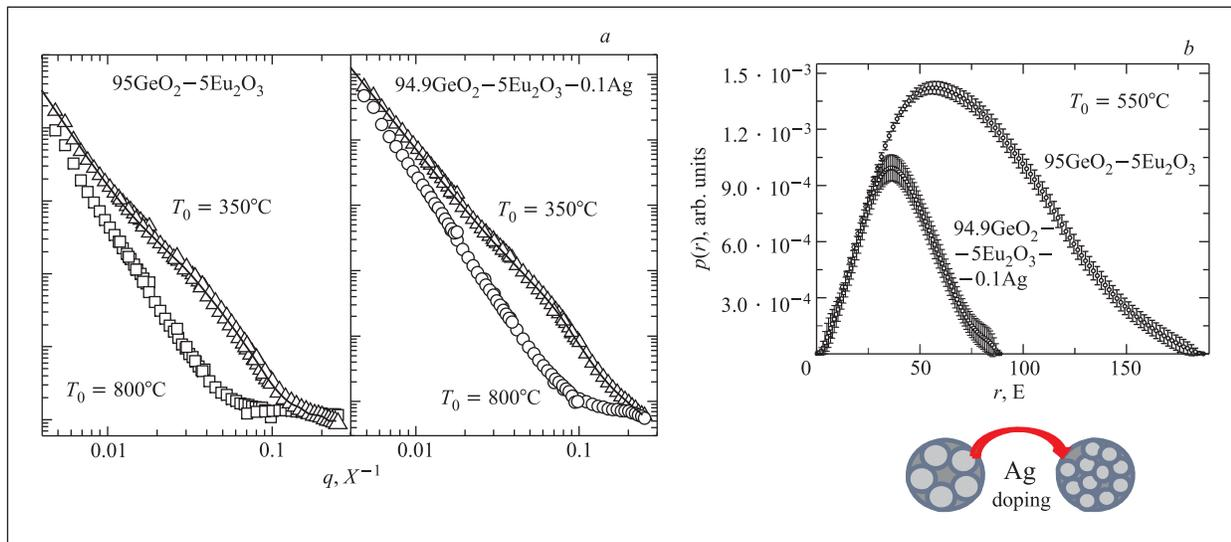
Fig. 1. *a*) Experimental and theoretical curves of small-angle neutron scattering of xerogels 95GeO<sub>2</sub>-5Eu<sub>2</sub>O<sub>3</sub> and 94.9GeO<sub>2</sub>-5Eu<sub>2</sub>O<sub>3</sub>-0.1Ag for annealing temperatures 350 and 500°C. *b*) Distribution function of intermediate aggregate sizes for xerogels 94.9GeO<sub>2</sub>-5Eu<sub>2</sub>O<sub>3</sub>-0.1Ag and 95GeO<sub>2</sub>-5Eu<sub>2</sub>O<sub>3</sub> for annealing temperatures 550°C
