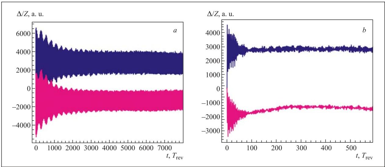
Fig. 1. Damping of horizontal injection errors (beam 1): damper OFF (a) and ON (b); signals from Q7 (top trace) and Q9 (bottom trace) pickups displaced by a quarter of the betatron oscillations' wavelength
