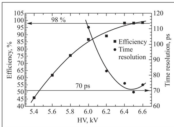
Fig. 5. RPC prototype efficiency and time resolution
