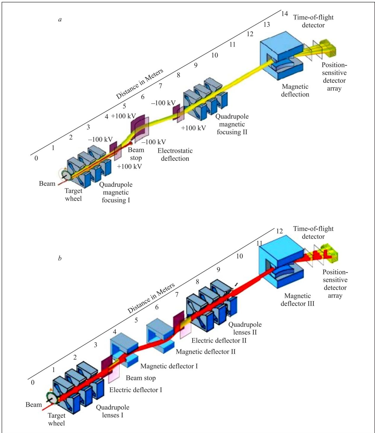
Fig. 2. Schematic view of the VASSILISSA separator before (a) and after (b) the upgrade
