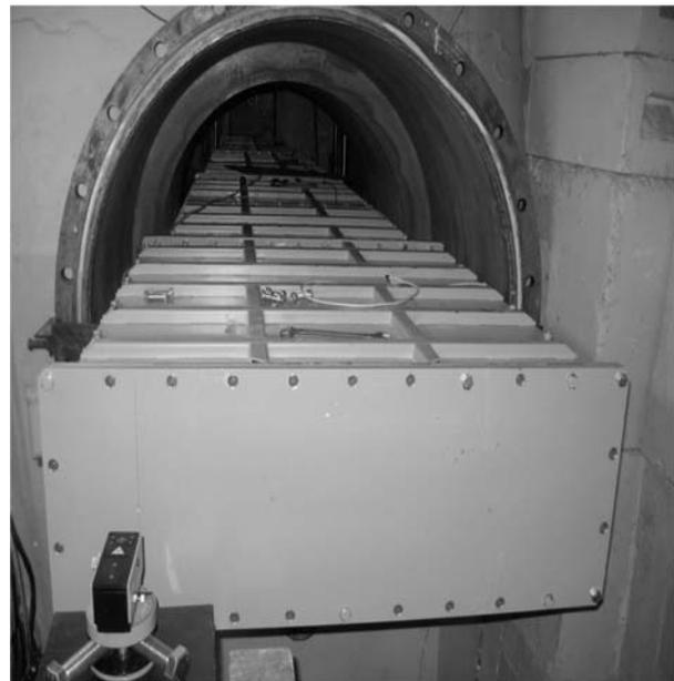
Fig. 2. The head part of the GRAINS reflectometer installed in the ring corridor of the IBR-2M reactor (Cooperation with Germany, Hungary, Romania)
