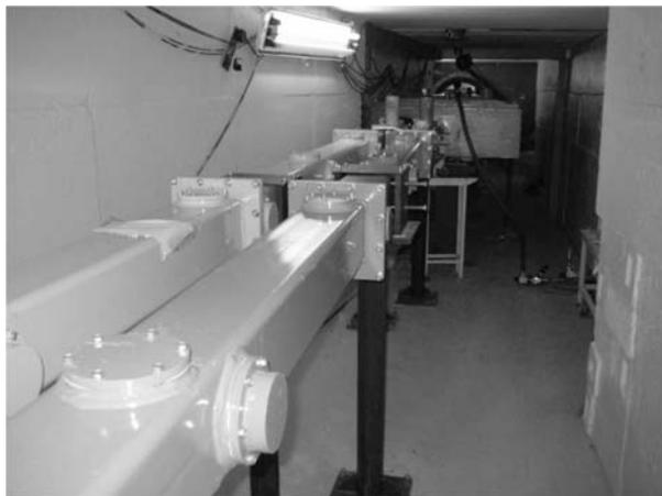
Fig. 4. First sections of curved neutron guides for EPSILON (left) and SKAT (right) (Cooperation with Germany)
