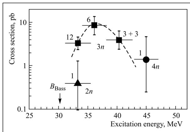
Fig. 2. Production cross sections of the nuclei  $^{289}_{115}$ ,  $^{288}_{115}$ , and  $^{287}_{115}$  vs. excitation energy of the compound nucleus. Figures show the number of the nuclei synthesized in the present experiment and in 2003
