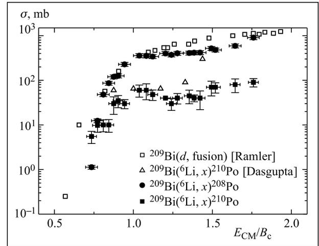
Fig. 4. Production cross sections for  ${}^{209}\text{Po}$  (●) and  ${}^{208}\text{Po}$  (■, △) vs.  $E_{\text{CM}}/B_c$  obtained in the reaction  ${}^6\text{Li} + {}^{209}\text{Bi}$ . Cross section for  ${}^{210}\text{Po}$  (□) from the reaction  ${}^{209}\text{Bi}(d, n){}^{210}\text{Po}$  is given for comparison
