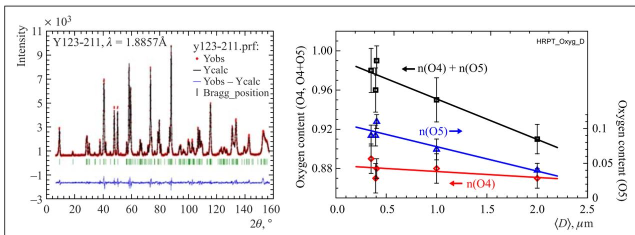
Fig. 1. Left: diffraction spectrum of YBa<sub>2</sub>Cu<sub>3</sub>O<sub>y</sub> sample (annealed at 930 °C with an average crystallite size  $\langle D \rangle = 2 \mu\text{m}$ ) obtained on HRPT (PSI, Switzerland) and treated by the Rietveld method. Right: site occupation factors for O(4) (left scale), O(5) (right scale) and their sum (left scale) as a function of the average crystallite size. Statistical errors of the points are indicated. Lines are drawn by the least squares method
