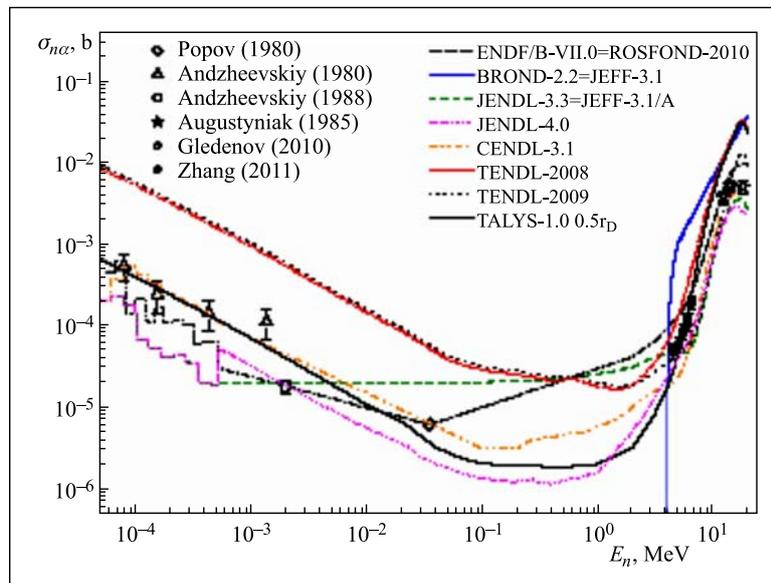
Fig. 3. Cross section of the  $^{149}\text{Sm}(n, \alpha)^{146}\text{Nd}$  reaction in comparison with the estimates available in the nuclear data libraries and the calculations performed using the TALYS-1.0 software package
