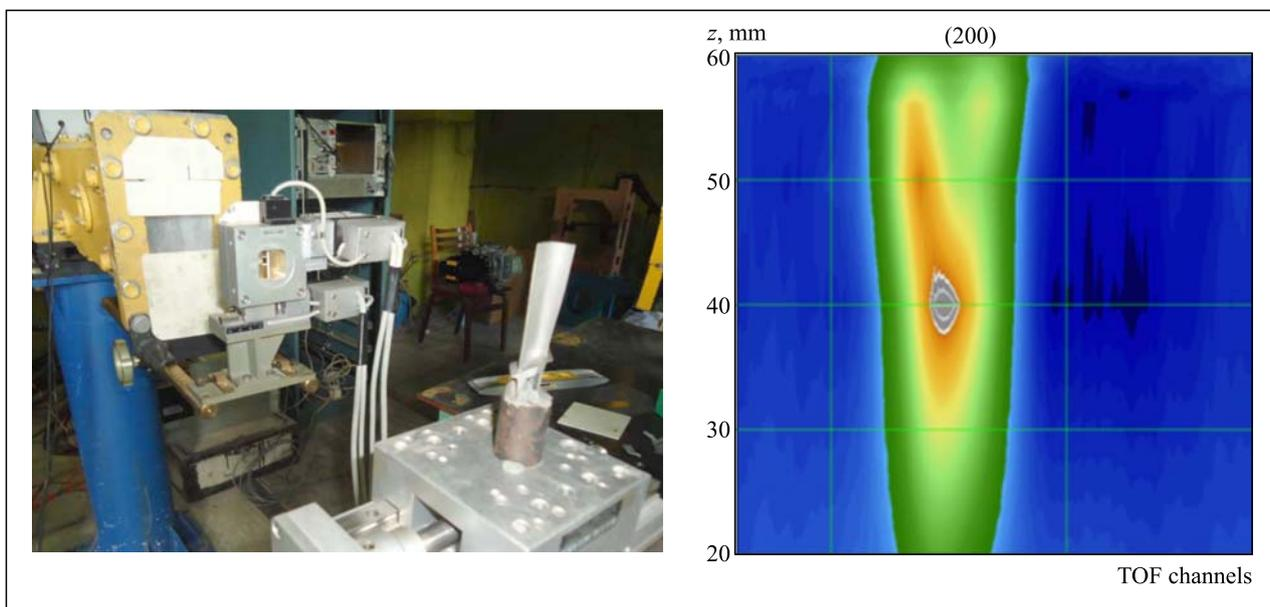
Fig. 2. Left: a turbine blade fixed on the goniometer of the FSD diffractometer for the experiment on the analysis of its microstructure. Right: 2D cross section of the region of the diffraction peak (200) revealing its complex topology. In particular, the presence of a grain with different (compared to the basic matrix) orientation can be seen
