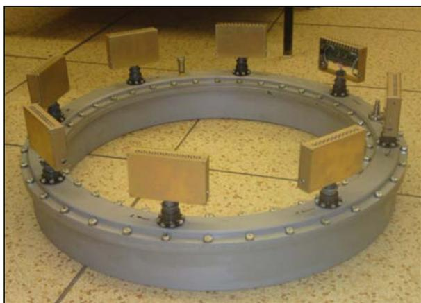
Fig. 4. The ring-shaped detector with 12-channel signal-shaping amplifiers mounted on its case
