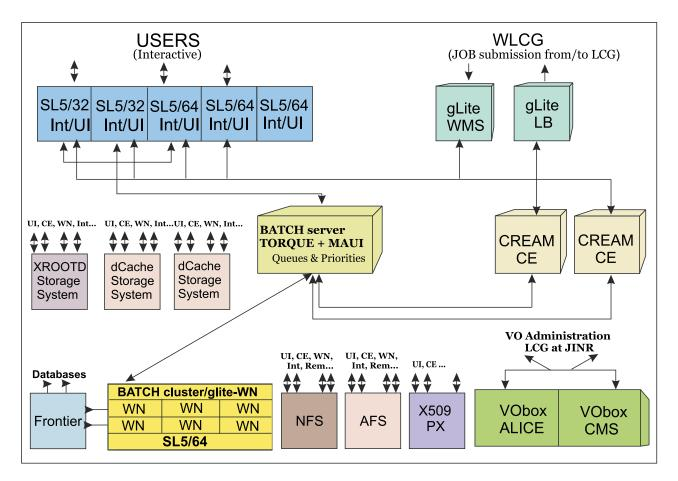
Fig. 2. A general scheme of the JINR CICC main components and their interoperation
