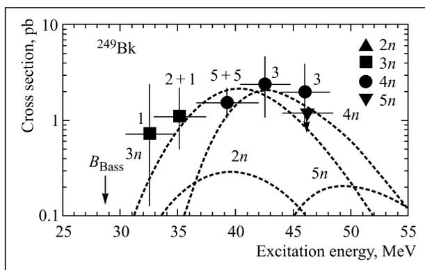
Fig. 2. Production cross sections of  $^{294}\text{117}$  and  $^{293}\text{117}$  vs. excitation energy of the compound nucleus. Figure specifies the number of nuclei synthesized in the present experiment and in 2010
