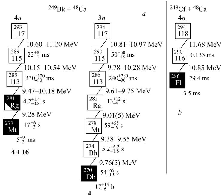
Fig. 1. (a) Radioactive properties of  $^{293,294}\text{117}$  and their daughter nuclei. Energies of  $\alpha$  particles and half-lives are given in the figure. The spontaneously fissioning isotopes are shown as black squares. (b) Decay chain of  $^{294}\text{118}$  (with  $\alpha$ -particle energies and decay times)
