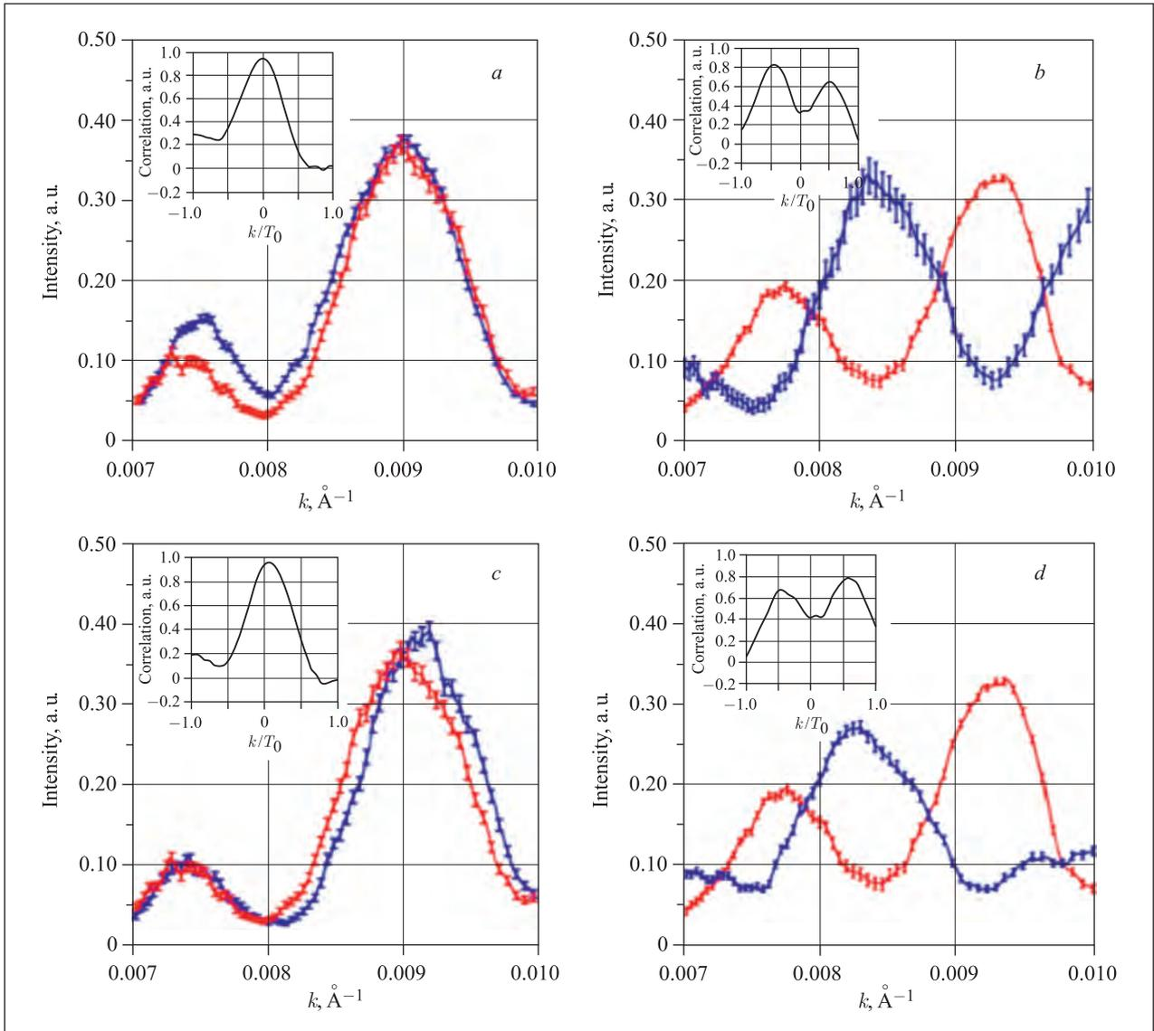
Fig. 2. The transmission for unpolarized neutrons obtained by using the first experimental scheme for CMS (a) and NCMS (b). The transmission of unpolarized neutrons obtained by using the second experimental scheme for CMS (c) and NCMS (d)
