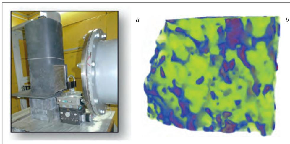
Fig. 3. *a*) Spectrometer for neutron radiography and tomography on IBR-2 beamline 14. *b*) Neutron tomographic image of the meteorite Seymchan showing the distribution of Fe–Ni alloy and fraction of rocks (mainly olivine)
