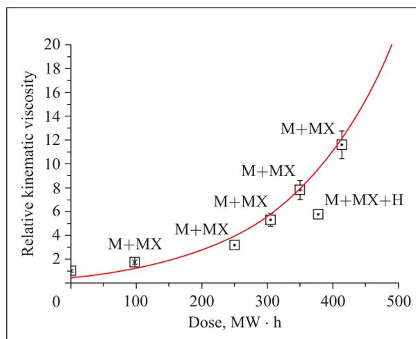
Fig. 4. Dependence of viscosity of the liquid mixture on the radiation dose: M + MX — mesitylene–metaxylene solution (in the ratio of 3:1), M + MX + H — solution of 55 g naphthalene dissolved in 1 liter of mesitylene–metaxylene mixture (in the ratio of 3:1)
