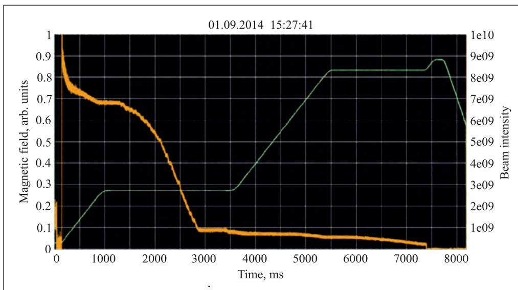
Fig. 1. The magnetic field cycle and beam intensity in the double user mode. At the first flat-top, the beam intensity decreases due to interaction with the internal target, at the second flat-top, the slow extraction is provided. At the both plateaus, RF is off
