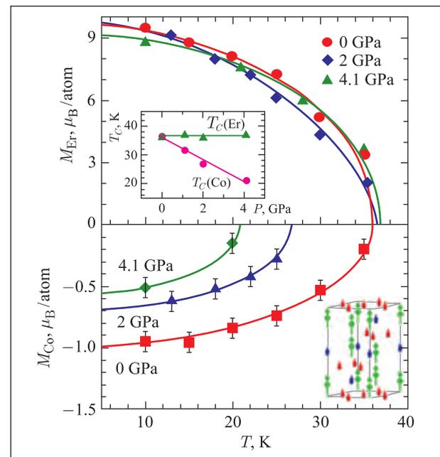
Fig. 1. Temperature dependences of Er and Co sublattice magnetizations in  $\text{ErCo}_2$  at different pressures, illustrating their independent behavior, which is beyond the IEM concept. The insets show the pressure dependences of the Curie temperatures of Er and Co sublattices and the character of the magnetic ordering in these compounds
