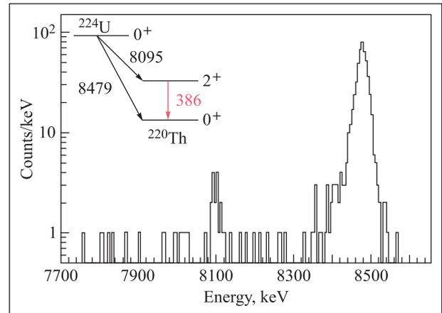
Fig. 3. Spectrum of  $\alpha$  decay of  $^{220}\text{Th}$
