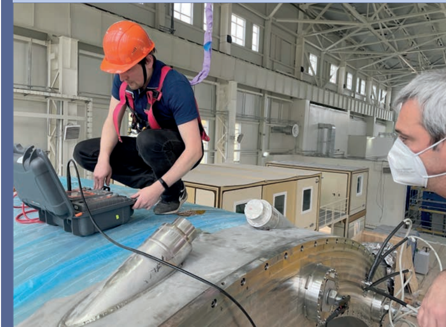
Testing the integrity of superconducting cables of the solenoid winding
