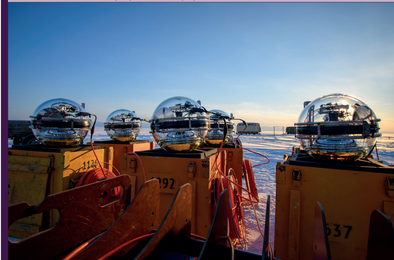
Baikal (Russia), March. Ice camp. Optical modules prepared for installation of the new cluster, the ninth one
