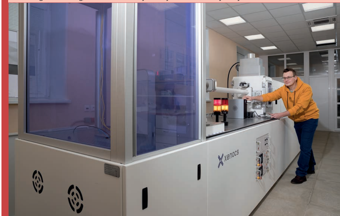
Xeuss 3.0 X-ray scattering station, which makes it possible to investigate nanoparticles using X-ray small-angle scattering, as well as to study the crystal structure by X-ray diffraction
