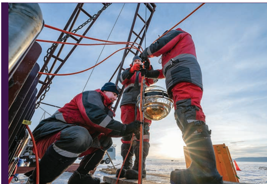
Lake Baikal, April. Installation of a garland of optical modules of the Baikal-GVD Neutrino Telescope
