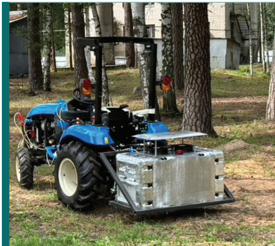
A scanner based on labeled neutrons (FLNP and Diamant) on an unmanned transport platform created at Dubna University
