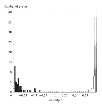
Fig. 6. Distribution of output signals from the neural network classifying noisy patterns with  $\sigma = 20$ . Threshold value is 0. Contribution of normal ECG patterns is presented by black histogram
