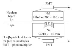
Fig. 1. Scheme of the total absorption spectrometer
