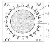
Fig. 5. The Kr2Det detector: *1*—the neutrino target (50 ton mineral oil + PPO); *2*—mineral oil; *3*—the transparent film; *4*—the PMTs; *5*—veto zone
