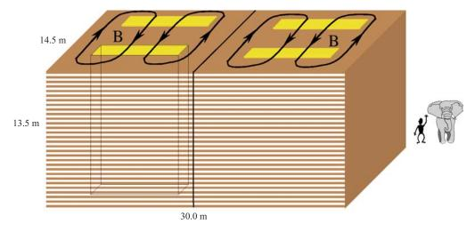
Fig. 1. Schematic view of the MONOLITH Detector. The arrangement of the magnetic field is also shown
