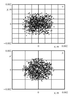
Fig. 18. Antiproton beam interaction with the helium target: a) diameter of beam spot at target location might be reduced to 2 mm; b) area in the phase space occupied by beam corresponds to recycler acceptance of  $A_x = 15 \pi \text{ mm} \cdot \text{mrad}$
