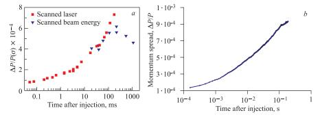
Fig. 14. Momentum spread of 18.4 keV/A Mg<sup>+</sup> beam as a function of time. The initial beam intensity is  $2.7 \cdot 10^{+7}$  ions: *a*) experimental data taken from [15]; b) BETACOOL simulations [37]. Due to intrabeam scattering, the r.m.s. momentum spread increases from around  $10^{-4}$  at injection up to  $7 \cdot 10^{-4}$  in about 150 ms
