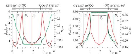
Fig. 5. Example of ELISA cell lattice starting at the middle of  $160^{\circ}$  deflector: *a*) ESD of spherical shape; *b*) ESD of cylindrical shape. The ring superperiodicity is 2. MAD-X simulations with electrostatic deflector matrixes [22]
