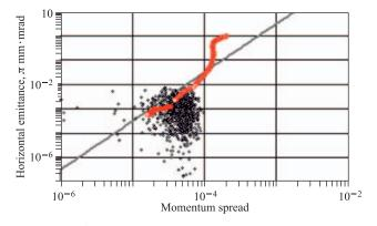
Fig. 29. Evolution of CF<sup>+</sup> beam distribution in 3D phase space ( $\Delta P/P$ ,  $\epsilon_x$ ). The centre of gravity of model beam presentation points corresponds to the equilibrium emittance of  $\epsilon_x^{eq} = 10^{-3} \pi \text{ mm} \cdot \text{mrad}$  and equilibrium momentum spread of ( $\Delta P/P$ )<sub>eq</sub> =  $5 \cdot 10^{-5}$
