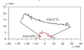
Fig. 6. Dynamic aperture of the ELISA storage ring with deflectors of cylindrical shape and ring with spherical deflectors. MAD-X nonlinear simulations [23]
