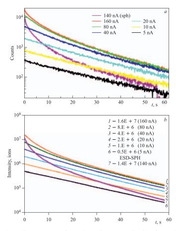
Fig. 3 (color online). Decays of stored negative oxygen O<sup>-</sup> ions in ELISA ring at 22 keV beam energy: *a*) experimental data taken from [15], beam lifetime  $\tau = 12$  s; *b*) BETACOOL simulations [34, 35]. Pink curve shows the drop of the beam current in ELISA ring with electrodes of spherical shape. The rest of the data related to ELISA ring are equipped with cylindrical electrodes
