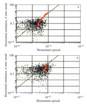
Fig. 34 (color online). Equilibrium distribution of 300 keV (*a*) and 20 keV (*b*) antiprotons in 3D phase space  $(\Delta P/P, \varepsilon_x)$  after electron cooling. Scattered points were simulated in the frame of the model beam algorithm [25]. Evolution of r.m.s. parameters during electron cooling is shown by red curve for 300 keV (*a*) and 20 keV (*b*) antiprotons
