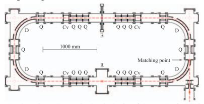
Fig. 15 (color online). Cross-sectional scale drawing of the recycler ring; horizontal cut including the mean path of the ion beam (dashed red line). Four  $90^{\circ}$  bending ES deflectors (D), four ESQ triplets (QQQ) and six ES single quads (Q) form ring lattice. Beam crosses gas jet in the reaction chamber (R)
