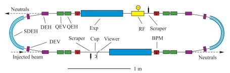
Fig. 2. Layout of ELISA storage ring taken from [14]. Ions are bent in  $10^{\circ}$  parallel plate deflectors (DEH) and  $160^{\circ}$  spherical deflectors (SDEH) and focused by electrostatic quads QEH and QEV. Neutrals might be detected after passing  $10^{\circ}$  parallel plate deflectors — DEH
