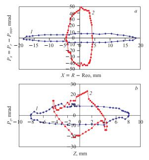
Fig. 8. Acceptance of ELISA ring [22]. Stable orbits have been tracked in relaxation electric field mesh generated by OPERA-3D/TOSCA software: *a*) radial phase space; *b*) vertical phase space. The middle of long straight section is marked as *I* and the middle of 160° deflector of cylindrical shape – as 2. Ring acceptance in vertical plane is less than  $30 \pi \text{ mm} \cdot \text{mrad}$
