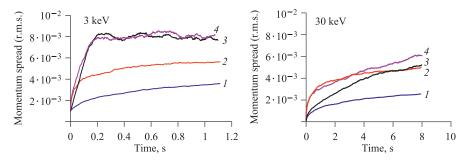
Fig. 19. Evolution of r.m.s. momentum spread of ions circulating in recycler ring. Target density is  $n_{\text{targ}} = 5 \cdot 10^{11} \text{ cm}^{-3}$ : *a*) ion energy is 3 keV; *b*) ion energy is 30 keV. Curves correspond to I — low beam intensity, target is OFF; 2 — high beam intensity, target is OFF; 3 — low beam intensity, target is ON; 4 — high beam intensity, target is ON
