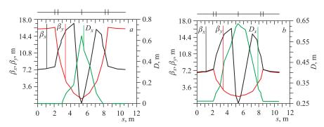
Fig. 31. Horizontal and vertical beta functions and dispersion of one ring quarter starting in the middle of long straight section: a) fourfold symmetry achromatic lattice; b) fourfold symmetry round beam mode. MAD-X simulations
