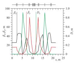
Fig. 32. An example of twofold symmetry achromatic lattice with low- $\beta$  functions at the ReMi location. One superperiod is shown. MAD-X simulations
