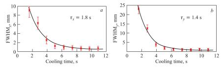
Fig. 24. Shrinking of the beam size in the TSR experiment on the transverse electron cooling of 93 keV/A CF<sup>+</sup> ions: *a*) equilibrium r.m.s. beam width in horizontal plane is  $\sigma_x = 0.2 \text{ mm}$ ; *b*) equilibrium r.m.s beam width in vertical plane is  $\sigma_y = 0.04 \text{ mm}$
