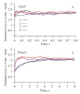
Fig. 17. Evolution of r.m.s. emittance of ions circulating in recycler ring. Target density is  $n_{\text{targ}} = 5 \cdot 10^{11} \text{ cm}^{-3}$ : *a*) ion energy is 3 keV; *b*) ion energy is 30 keV. Curves correspond to I — low beam intensity, target is OFF; 2 — high beam intensity, target is OFF; 3 — low beam intensity, target is ON; 4 — high beam intensity, target is ON
