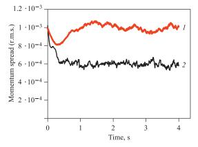
Fig. 37. Evolution of momentum spread (r.m.s.) of high intensity beam of 20 keV antiprotons cooled down by electron gun with thermocathode (*I*) and with photocathode (2). Equilibrium momentum spread is  $(\Delta P/P)_{\rm rms}^{\rm eq} = 10^{-3}$  and  $(\Delta P/P)_{\rm rms}^{\rm eq} = 6 \cdot 10^{-4}$ , respectively
