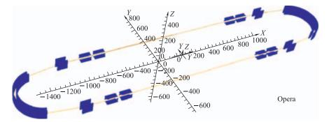
Fig. 4. Model of the ELISA ring in OPERA-3D. The dimensions and distances were taken from [4, 13]. Particles were tracked over many turns in order to find stable solution for closed equilibrium orbit
