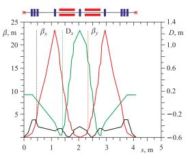
Fig. 16 (color online). Example of beta-functions and dispersion for the recycler ring (MAD-X simulations). One cell starting in the middle of long straight section is shown. In the interaction points the low-beta mode is realized ( $\beta_{x,y} \leq 10$  cm), also dispersion is varied to the achromatic conditions (D = D' = 0)
