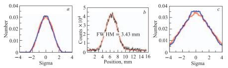
Fig. 9. Beam profile of 18.4 keV Mg<sup>+</sup> ions in ELISA ring with spherical deflectors: a) BETACOOL simulations correspond to the ring acceptance of  $A \sim 6\pi$  mm · mrad ( $\sigma = 1.5$  mm); b) experiment curve taken from [15] corresponds to the ring acceptance  $\sim 5\pi$  mm · mrad ( $\beta_x = 3.5$  m); c) expected beam profile assuming the ring acceptance would be  $\sim 50\pi$  mm · mrad
