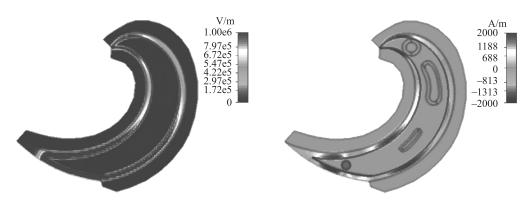
Fig. 9. Electric field distribution
