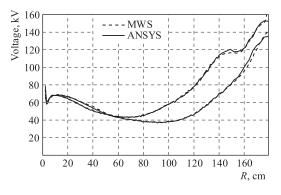
Fig. 8. Voltage distribution along radius
