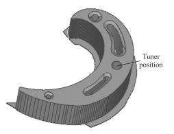
Fig. 7. View of the ANSYS model with tuner
