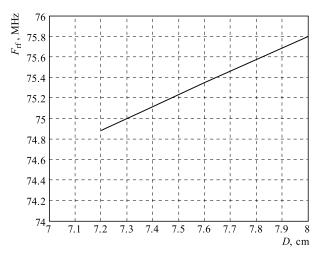
Fig. 11. Frequency of the cavity against diameter of the fourth stem
