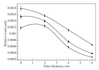
Fig. 8. Relative yield of selected dp events as a function of the filter thickness:  $\blacktriangle$  — criteria A;  $\blacksquare$  — criteria A+B;  $\blacktriangledown$  — criteria A+B with the background subtraction (curves are presented for better visualization)
