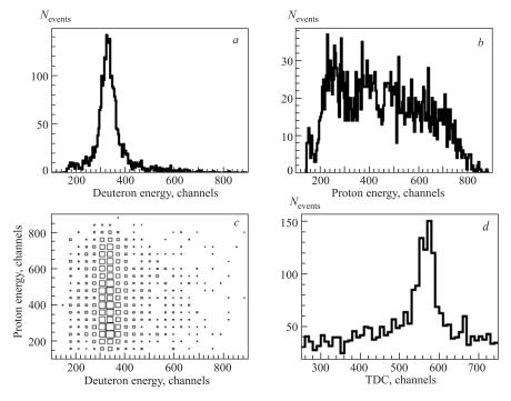
Fig. 4. The results obtained at 2.0 GeV deuteron beam on carbon target: a) deuteron energy losses; b) proton energy losses; c) correlation of proton and deuteron energy losses; d) time difference between the signals for deuteron and proton detectors
