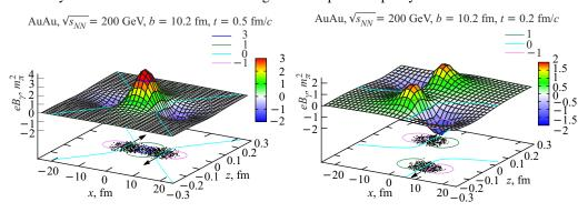
Fig. 4. Distribution of the magnetic field strength  $eB_y$  in the y=0 plane at t=0.05 (a) and 0.2 (b) (in the middle) fm/c for Au + Au collisions at  $\sqrt{s_{NN}} = 200$  GeV and b = 10.2 fm. The collision geometry is projected on x-z plane by points corresponding to a particular spectator position. Curves (and their projections) are levels of the constant  $eB_y$
