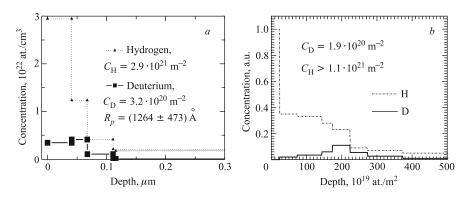
Fig. 14. The depth concentrations of D and H atoms after D<sup>+</sup>-ion implantation with the energy of 25 keV at a fluence of  $\Phi_1 = 1.2 \cdot 10^{22} \text{ m}^{-2}$  in  $Pd_{0.9}Rh_{0.1}$  samples 10 days after (a) and three month later (b)
