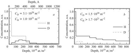
Fig. 10. ERDA depth concentrations of D and H atoms after implantation of D<sup>+</sup> ions up to a fluence of  $\Phi = 1.2 \cdot 10^{22} \text{ m}^{-2}$  (a) and saturation under 9 kbar deuterium gas during three days of  $Pd_{0.9}Ag_{0.1}$  sample (b). Measurements were carried out three months after implantation and saturation
