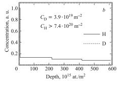
Fig. 2. The experimental and simulated spectra of H and D recoils measured by ERDA (a) and calculated depth concentrations of D and H atoms after saturation of Pd<sub>0.9</sub>Ru<sub>0.1</sub> alloy under 9 kbar deuterium gas high pressure during 72 h (b). Measurements were carried out a long period of time after saturation
