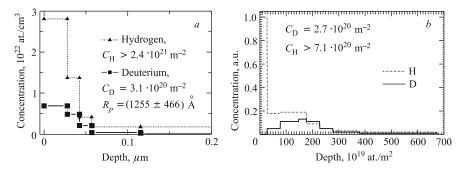
Fig. 15. The depth concentrations of D and H atoms after D<sup>+</sup>-ion implantation with the energy of 25 keV at a fluence of  $\Phi_1 = 1.2 \cdot 10^{22} \text{ m}^{-2}$  in  $Pd_{0.9}Ru_{0.1}$  samples 10 days after (a) and three month later (b)
