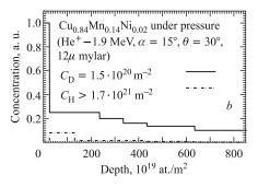
Fig. 3. The experimental and simulated spectra of H and D recoils measured by ERDA (a) and calculated depth concentrations of D and H atoms after saturation of manganin alloy sample under 9 kbar deuterium gas high pressure during 72 h (b). Measurements were carried out a long period of time after saturation
