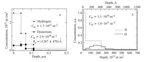
Fig. 12. The depth concentrations of D and H atoms after D<sup>+</sup>-ion implantation with the energy of 25 keV at a fluence of  $\Phi_1 = 1.2 \cdot 10^{22} \text{ m}^{-2}$  in  $Pd_{0.9}Ag_{0.1}$  samples 10 days after (a) and three months later (b)
