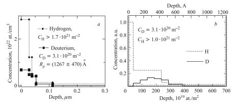
Fig. 13. The depth concentrations of D and H atoms after D<sup>+</sup>-ion implantation with the energy of 25 keV at a fluence of  $\Phi_1 = 1.2 \cdot 10^{22} \text{ m}^{-2}$  in Pd<sub>0.9</sub>Pt<sub>0.1</sub> samples 10 days after (a) and three months later (b)
