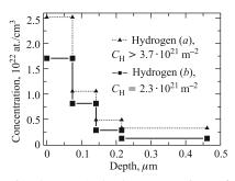
Fig. 5. ERDA depth concentrations of D and H atoms in manganin samples: annealed sample (at 125 °C, one hour) — histogram (a) and without annealing — histogram (b)
