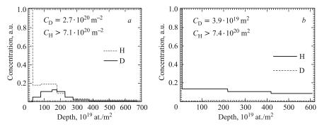
Fig. 9. ERDA depth concentrations of D and H atoms after implantation of  $D^+$  ions up to a fluence of  $\Phi = 1.2 \cdot 10^{22} \text{ m}^{-2}$  (a) and saturation under 9 kbar deuterium gas during three days of  $Pd_{0.9}Ru_{0.1}$  sample (b). Measurements were carried out 30 days after saturation and implantation
