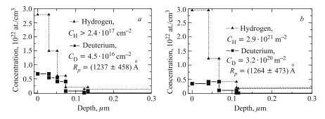
Fig. 11. The depth concentrations of D and H atoms after implantation of D<sup>+</sup> ions with the energy of 25 keV at a fluence of  $\Phi_1 = 1.2 \cdot 10^{22} \text{ m}^{-2}$  in pure Pd (a) and Pd<sub>0.9</sub>Ag<sub>0.1</sub> (b) samples
