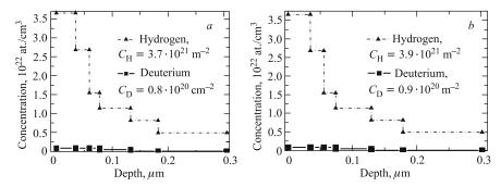
Fig. 4. ERDA depth concentrations of D and H atoms after saturation of annealed manganin sample (at  $125\,^{\circ}$ C, one hour) under 9 kbar deuterium gas high pressure during 72 h. Measurements were carried out one month after saturation on the same sample just in different places ((a) and (b)) for detailed comparison of result repetition
