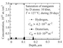
Fig. 6. ERDA depth concentrations of D and H atoms after saturation of annealed (at 125 °C, one hour) manganin sample under 10 kbar deuterium gas high pressure during twenty days at 127 °C temperature. Measurements were carried out 5 days after saturation
