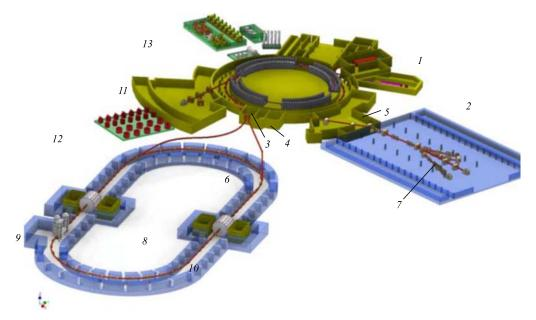
Fig. 1. Scheme of the NICA facility: 1 - light and polarized ion sources and «old» Alvarez-type linac; 2 - ESIS source and new RFQ linac; 3 - Synchrophasotron yoke; 4 - booster; 5 - Nuclotron; 6 - beam transfer lines; 7 - Nuclotron beam lines and fixed target experiments; 8 - collider; 9 - MPD; 10 - SPD; 11 - new research area; 12 - cryogenic plant; 13 - auxiliary equipment
