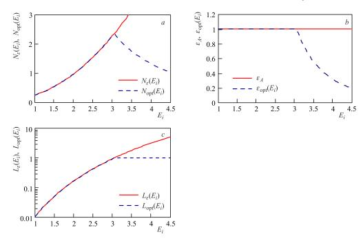
Fig. 2. Space charge dominated regime; ion number per bunch (*a*), emmitance (*b*) and luminosity (*c*) versus ion energy in two cases: full acceptance if filled with ions (red solid curve) and luminosity is limited (blue dashed curve); the ring acceptance =  $40 \pi \cdot \text{mm} \cdot \text{mrad}$ , parameter units:  $[N_i] = 10^9$ ,  $[\varepsilon] = \pi \cdot \text{mm} \cdot \text{mrad}$ ,  $[L] = 10^{27} \text{ cm}^{-2} \cdot \text{s}^{-1}$
