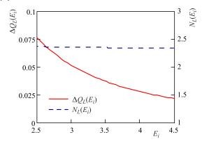
Fig. 3. IBS dominated regime; beam tune shift  $\Delta Q_{\text{tot}}$  (red solid curve) and ion number per bunch  $N_i$  (blue dashed curve) at constant luminosity  $L = 1 \cdot 10^{27} \text{ cm}^{-2} \cdot \text{s}^{-1}$  and beam emittance of 1.0  $\pi \cdot \text{mm} \cdot \text{mrad}$ ;  $[N_i] = 10^9$
