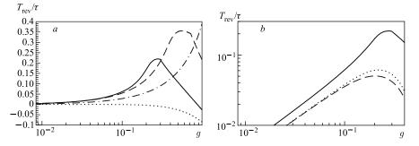
Fig. 4. Dependences of  $T_{\rm rev}/\tau$  on gain g for H(z) = 1 (dash-dotted),  $H_N(z)$  (dotted),  $H_1(z)$  (solid),  $H_2(z)$  (dashed) in the panel a and for TFS with  $H_1(z)$  at  $\Delta \varphi = -116.4^\circ$  (solid),  $\Delta \varphi = -76.4^\circ$  (dashed),  $\Delta \varphi = -156.4^\circ$  (dotted) in the panel b
