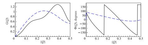
Fig. 2. The magnitude G(Q) and phase response  $\Phi(Q)$  graphs for the notch and Hilbert filters (solid) and for the notch filter and the FIR filter of the first order (dashed)
