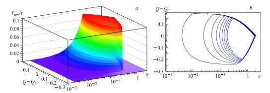
Fig. 1. Beam stability surface (a) and contour (b) plots
