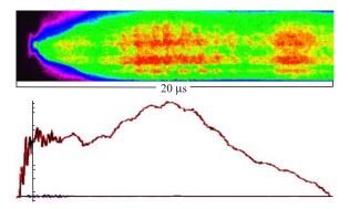
Fig. 3. Time scanning of the discharge luminescence and current for long pulse mode
