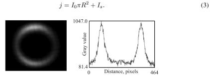
Fig. 6. Light output from scintillator and the density distribution of ion Fe<sup>+26</sup> at 1.7  $\mu$ s after beginning of discharge at a distance of 30 cm for a current of 150 kA. The ring diameter is 9 mm
