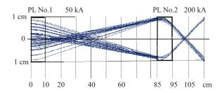
Fig. 9. Formation of a converging conic beam by means of two plasma lenses
