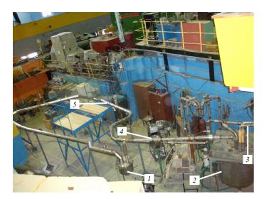
Fig. 2. The full-scaled model of the conveying path and the technological system of the IBR-2M cryogenic moderator installed at the experimental hall of the IBR-2 reactor: 1 — the chamber-imitator of the cryogenic moderator; 2 — the cryostat (with the heat exchanger and the helium blower inside); 3 — the cryogenic pipeline from/to the refrigerator; 4 — the charging device; 5 — the cryogenic pipeline for conveying mesitylene beads
