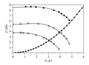
Fig. 4. Flow rate-pressure drop relation of the helium blower at some values of the blower rotation speed: squares — 22 500 rev./min, circles — 18 000 rev./min, void triangles — 15 000 rev./min; solid triangles — hydrodynamic resistance of the conveying pipe
