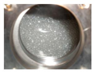
Fig. 3. Photo of the cold solid beads of mesitylene at  $T \sim 40$  K inside the chamber-imitator of the moderator chamber
