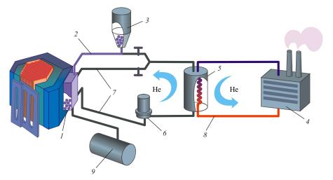
Fig. 1. The pelletized cold moderator and its operating principle at the IBR-2M reactor: 1 - cold moderator; 2 - charging pipeline; 3 - charging device; 4 - helium refrigerator; 5 - heat exchanger; 6 - helium blower; 7 - primary helium loop; 8 - secondary helium loop; 9 - used mesitylene receiver
