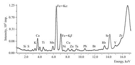
Fig. 1. XRF spectrum of coal sample
