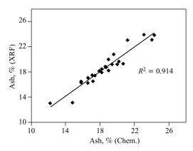
Fig. 3. Comparison of ash contents determined by XRF technique and conventional techniques
