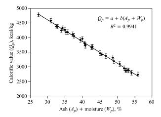
Fig. 5. Correlation between the calorific value and the sum of coal ash and moisture content by reference coal samples
