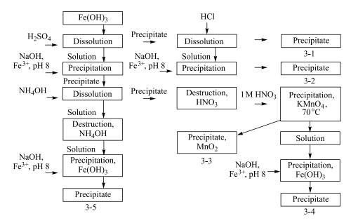
Fig. 3. The scheme of iron hydroxides processing from the cube residue (2-1)
