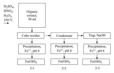
Fig. 2. The scheme of the processing of the extract
