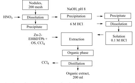
Fig. 1. The scheme of hydrochemical processing of 13 kg iron-manganese nodules from the 6298-52 station
