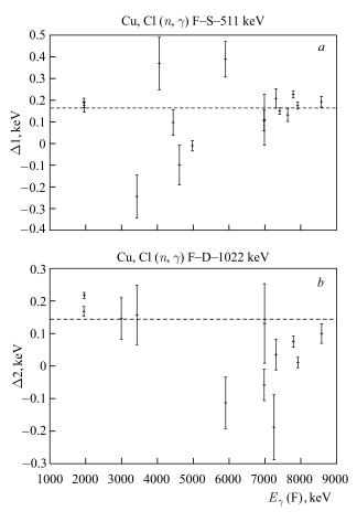
Fig. 5. Dependence of distances  $\Delta 1 = E_{\rm F} - E_{\rm S} - 511$  keV (a) and  $\Delta 2 = E_{\rm F} - E_{\rm D} - 1022$  keV (b) on  $E_{\gamma}({\rm F})$ . The mean values are shown by lines
