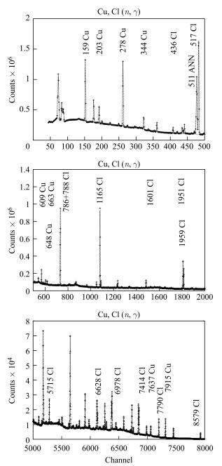
Fig. 4. Three parts of spectrum Cu,  $\mathrm{Cl}(n,\gamma)$  with peaks which were used in calibration procedure
