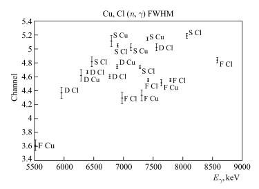
Fig. 3. Dependence of FWHM on  $E_{\gamma}$ . Single escape (S), double escape (D) and full energy (F) peaks are indicated
