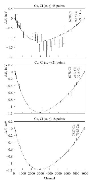
Fig. 6. Deviation of the energy calibration function from a linear one. Three variants of selected points and obtained calibration curves are given
