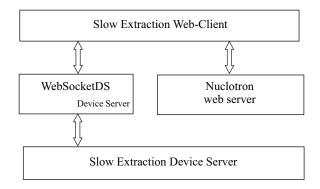
Fig. 5. Interconnection diagram of the Slow Extraction Control Web-Client
