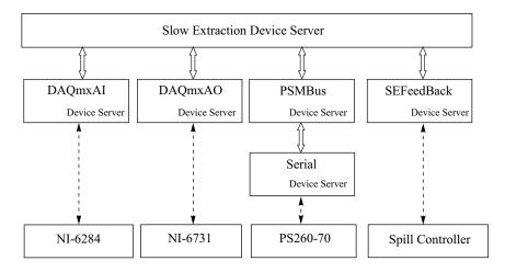
Fig. 3. Diagram of the equipment control by the Slow Extraction Device Server
