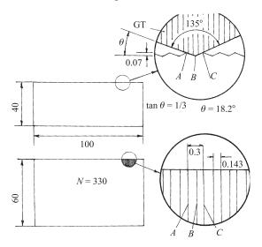
Fig. 3. Image orthogonalization system: GT — grooving tool; A, B and C are three points of the lamelar region; BC is the working part of the lamelar mirror. All dimensions are in millimetres
