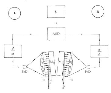
Fig. 5. Coincidence electronic circuit for two output signals from the stereoscopic confocal scanner for vertical particle tracks:  $M_3$  — two orthogonalization mirrors; PhD — two point-like photodiodes; d/dt — time differentiation circuit; AND — coincidence electronic circuit; S — storage block
