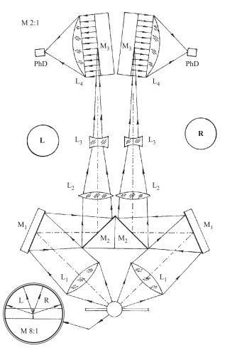
Fig. 4. Stereoscopic confocal scanner for the vertical particle tracks, provided with two confocal scanners on both sides of view (L and R):  $L_1$  — two main imaging lenses;  $L_2$  and  $L_3$  — two pairs of Newton monocular lenses;  $L_4$  — two collecting lenses;  $M_1$  — two first-plane mirrors;  $M_2$  — two second-plane mirrors;  $M_3$  — two orthogonalization mirrors; PhD — two point-like photodiodes
