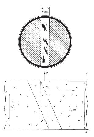
Fig. 1. The results of the experimental testing of the dark-field confocal scanning microscope for selective observation of the vertical particle tracks [4]. *a*) Signals of four particle tracks inside the illuminating zone of  $6 \,\mu\text{m}$  width. *b*) The cross section of the same region
