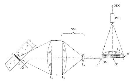
Fig. 2. The principal scheme of the confocal scanner for vertical particle tracks:  $L_1$  — main imaging lens;  $L_2$  and  $L_3$  — lenses of the Newton monocular;  $L_4$  — collecting lens; OM — orthogonalization mirror; PhD — point-like photodiode; A', O' and B' are the imaging points of A, O and B points of the vertical particle track; d — width of the illuminating zone,  $\sim 2 \mu m$
