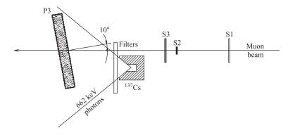
Fig. 2. Experiment layout (top view)
