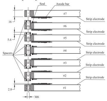
Fig. 1. P3 cross section
