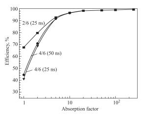
Fig. 7. The CSC efficiency vs. absorption factor for 25 and 50 ns strobe widths
