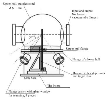
Fig. 1. Scheme of the internal target station
