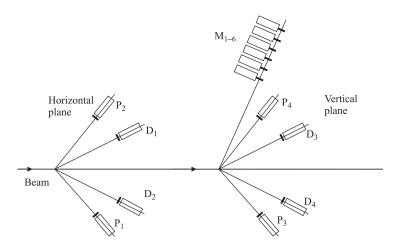
Fig. 3. Scheme of the detectors. P and D are the scintillation counters for the detection of the proton and deuteron, respectively;  $M_{1-6}$  are the monitor scintillation counters
