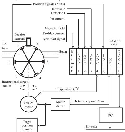
Fig. 2. Block scheme of the internal target station control and target position monitor
