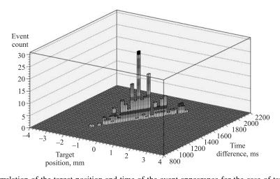
Fig. 6. Correlation of the target position and time of the event appearance for the case of target moving in the direction from the accelerator ring center
