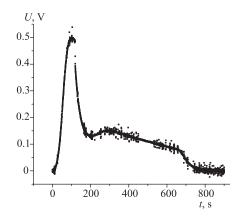
Fig. 6. The time dependence of structure decay in kerosene-based magnetic fluid without additional illumination
