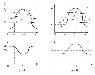
Fig. 2. The illustration of particle thermodiffusion in disperse fluid with positive S > 0 and negative S < 0 thermodiffusion coefficient, respectively
