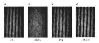
Fig. 5. The grating decay in kerosene-based magnetic fluid without (a, b) and with (c, d) additional illumination
