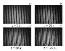
Fig. 3. The shifted interference and concentration gratings in kerosene-based magnetic fluid with S<0
