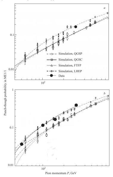
Fig. 11. Punch-through probability vs pion beam energy for EE + HE + ME1/1 (a) and HE + ME1/1 (b) configurations. Simulation for four GEANT4 models considered is given for extended region up to 1 TeV/c
