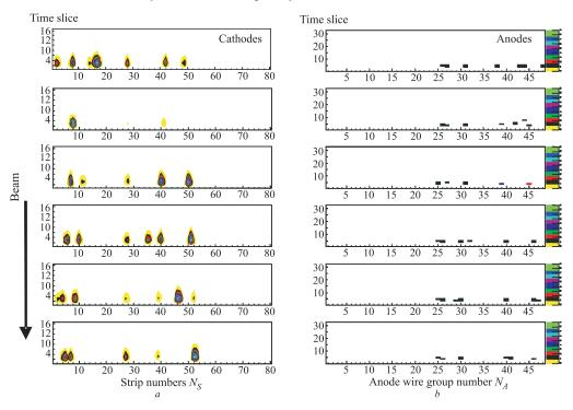
Fig. 5. The experimental event with punch-through in ME1/1' (pion with energy of 300 GeV)
