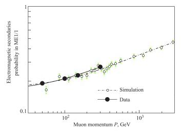
Fig. 10. Electromagnetic secondaries probability in ME1/1 vs muon beam energy. Simulation for four GEANT4 model lists is given for extended region up to 3 TeV/c
