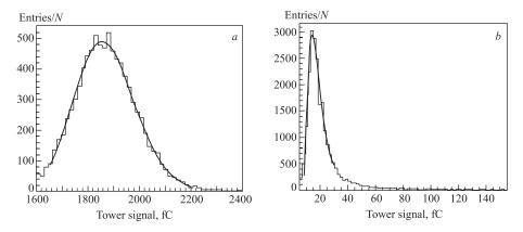
Fig. 6. Amplitude spectra for pions (a) and for muons (b) in HE towers for beam energy of 300 GeV. For pions the signal is from a  $3\times3$  matrix of towers, or muons from a single tower
