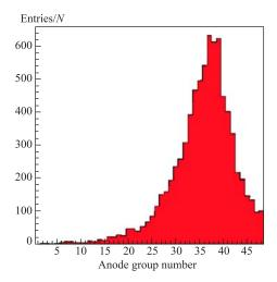
Fig. 9. ME1/1' anode filling histogram for 300 GeV pion beam (the width of the anode group is 2.7 cm)
