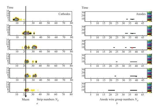
Fig. 3. Experimental event with electromagnetic secondaries in ME1/1' (300 GeV muons)
