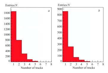
Fig. 8. Track number distribution for punch-through events in ME1/1' for HE + ME1/1' (a) and EE + HE + ME1/1' (b)
