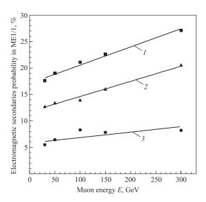
Fig. 4. Electromagnetic secondaries probability in ME1/1' vs muon beam energy.  $\blacksquare$ , l - ME1/1 mounted on HE (separate and distorted clusters);  $\blacktriangle$ , 2 - ME1/1 behind magnet (separate and distorted clusters);  $\bullet$ , 3 - ME1/1 mounted on HE (secondaries from HE)
