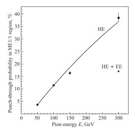
Fig. 7. The punch-through probability vs pion beam energy for the HE + ME1/1 configuration (solid line, circles) and for the HE + EE + ME1/1 configuration (square)
