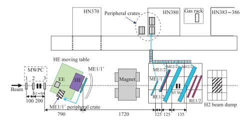
Fig. 1. The experimental set-up (distances given in cm). Length of optical links from peripheral crates — 50 m; counters: S1, S4 —  $14 \times 14$  cm; S2 —  $4 \times 4$  cm; S3 —  $2 \times 2$  cm; S5 —  $10 \times 10$  cm; S6 —  $12 \times 12$  cm
