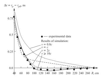
Fig. 2. Measured values of the difference,  $\Delta t$ , between the first zero crossing times of the signals  $\epsilon_v(t)$  and  $\epsilon^{\rm ref}(t)$ , in comparison with simulations for different values of v from [15]. The measurement error on each experimental datum is  $\simeq 0.02$  ns. The prediction v=c of conventional CEM is completely excluded whereas the data are consistent with the QED prediction  $v=\infty$  which is indistinguishable from the  $v\geqslant 10c$  curve shown
