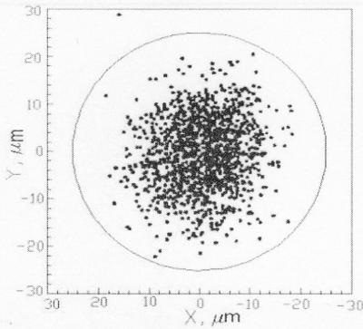
Fig. 11: Results of Roentgen test of aluminium tubes are given (scatter plot) in the form of a measured deviation of the location of a signal wire from the centre of the tube. The circle with a radius of  $24 \mu\text{m}$  presents the limit for the deviations allowed by the required quality.
