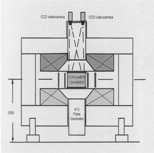
Fig. 20: Sketch of the DUBTO Streamer chamber ( $47 \times 60 \times 16 \text{ cm}^3$ ) in the magnet MC-4A ( $B = 0.690 \pm 0.005 \text{ T}$ ).
