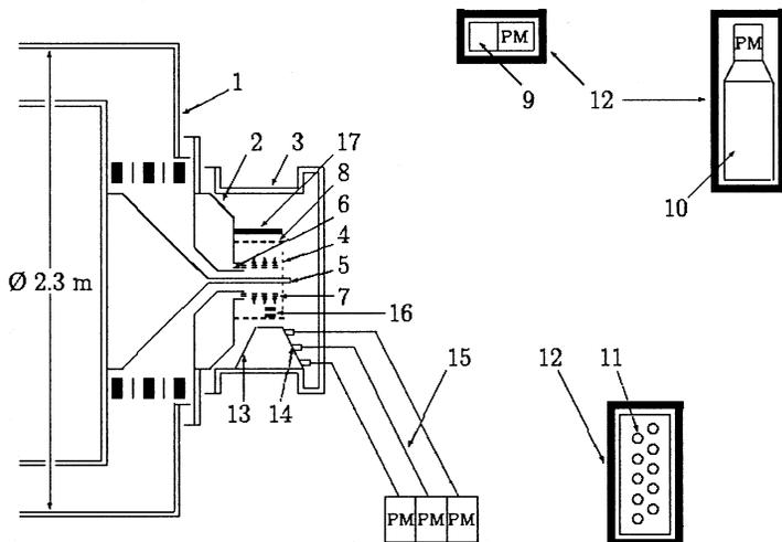
Fig. 34: 1 — high current generator, 2 — load unit, 3 — diagnostic chamber, 4 — wire mesh cathode, 5 — return current rod; 6 — supersonic Laval nozzle, 7 — liner, 8 — current-intercepting squirrel cage, 9 — scintillation detector I, 10 — scintillation detector II, 11 — thermal neutron detector, 12 — Pb shielding, 13 — cone, 14 — collimator, 15 — light guide, 16 — B-dot probe, 17 — CD polymer target, PM — photomultiplier.
