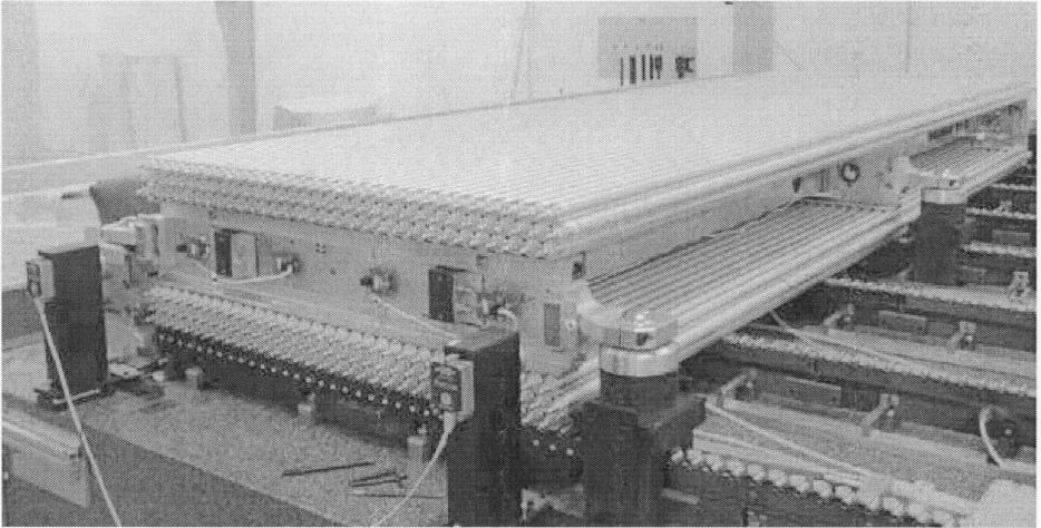
Fig. 12: Drift chamber BMS-5 is settled on the granite table after complete gluing of 6 layers of drift tubes (3 layers are under the supporting farm and 3 layers are above the farm). The chamber is held by side blocks by means of spherical piers. In the foreground one can see the elements of the optical system for outer (two towers) and inner (4 blocks of lightdiodes) adjustment.
