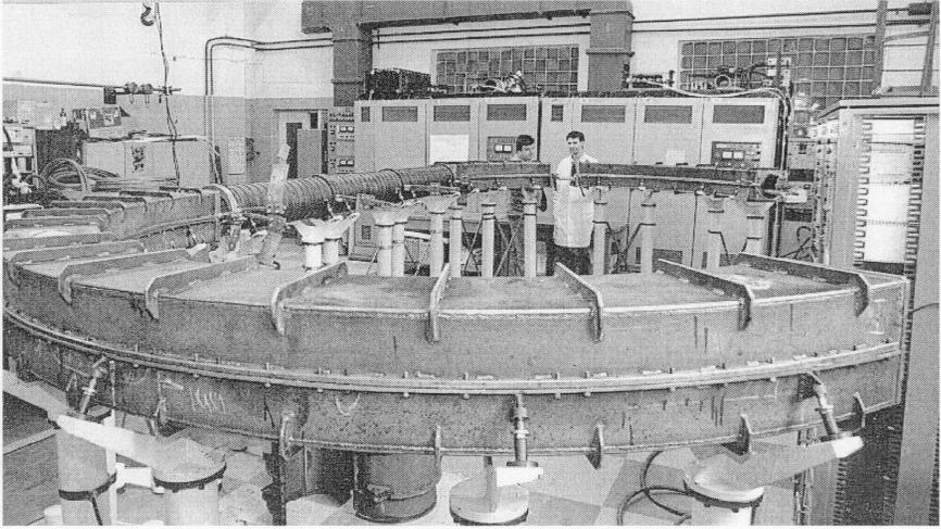
Fig. 36: Magnetic system of LEPTA.
