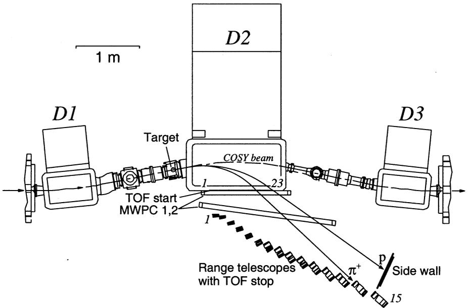
Fig. 26: The layout of magnetic the spectrometer ANKE.
