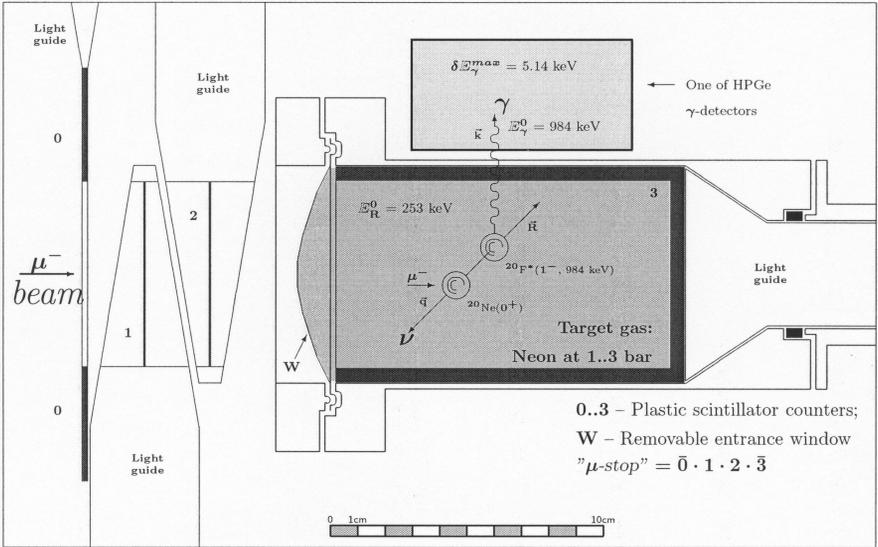
Fig. 33: Set-up with gaseous Ne.
