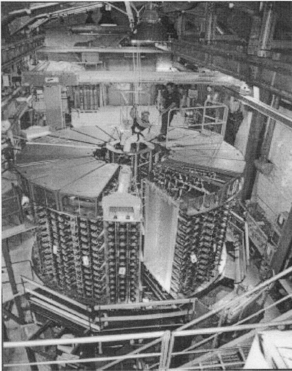
Fig. 32: Spectrometer NEMO-3 at the end of its construction: the 19th sector is being mounted.
