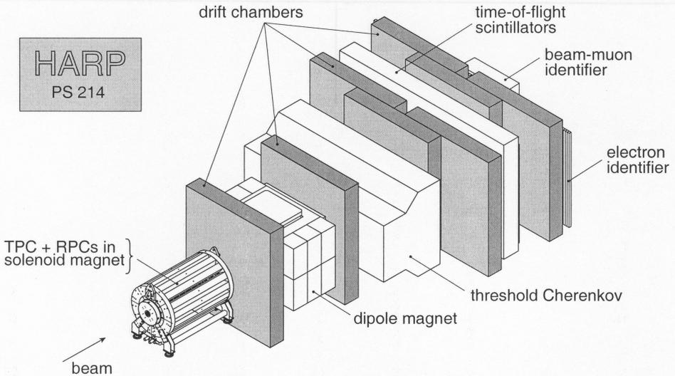
Fig. 19: Layout of the HARP experiment.
