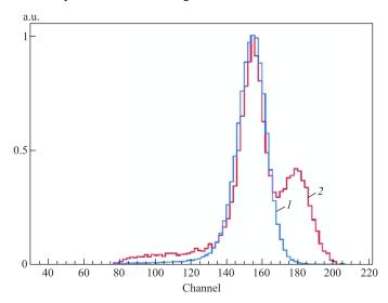
Fig. 4. Amplitude spectrum of the signals recorded by an  $\alpha$  pixel without coincidence with the signal from the gamma detector
