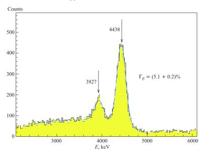
Fig. 6. Energy spectrum of  $\gamma$  rays recorded by the gamma detector in irradiation of a  $^{12}{\rm C}$  sample with a tagged neutron flux
