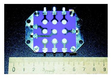
Fig. 2. Nine-pixel alpha detector viewed from the back
