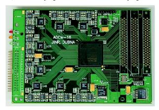
Fig. 7. The data acquisition board with 16 channels for alpha and gamma detector signals
