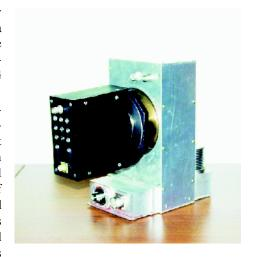
Fig. 3. The box of the frontend electronics of the alpha detector mounted on a neutron generator with ground target
