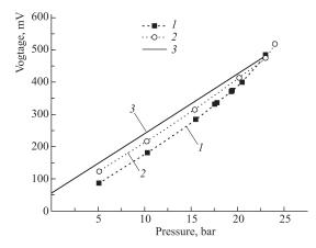
Fig. 4. Response of the displacement gauge to the gas pressure load on the membrane at 70–80 K. Curve 1 is for the first load after heating up to room temperature, curve 2 is for the second load, and curve 3 — for the third load and the following
