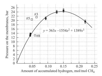
Fig. 7. Peak value of pressure during heating of irradiated methane versus amount of hydrogen accumulated. Black squares — experiments with the normal amount of methane in the chamber and with medium or high rate of heating; hollow squares — experiments with different parameters of heating
