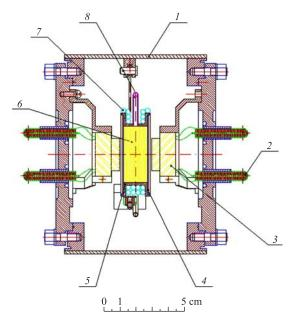
Fig. 3. Evacuated chamber with a sample, elevation along diameter. 1 - cylindrical shell of the chamber; 2 - coaxial cables of displacement gauges (3); 4 - steel membrane; 5 - steel shell of a sample chamber; 6 - the sample (aluminium sponge filled with solid methane); 7 - coil of copper tube (heat exchanger); 8 - steel tube for filling and evacuation of methane and hydrogen gases
