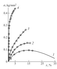
Fig. 11. Uniaxial tensile stress-strain curves  $\sigma$  at the deformation rate  $d\varepsilon/dt = 3.3 \cdot 10^{-4} \text{s}^{-1}$  on a polycrystal CH<sub>4</sub>: 1) T = 77 K; 2) T = 64 K; 3) T = 20 K; 4) T = 4.2 K
