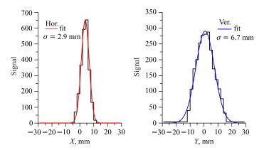
Fig. 4. The X- (left) and Y- (right) coordinate beam profile at the focus F5. The lines are the same as in Fig. 7
