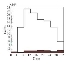
Fig. 6. The X-coordinate beam profile measured by scintillation hodoscope. The open and dashed histograms are the carbon and single charged particles, respectively
