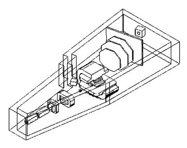
Fig. 1. The 6V beamline with GIBS magnet in building 205, consisting of the doublet of quadrupole magnets, two small dipole magnets and large-aperture magnet SP41
