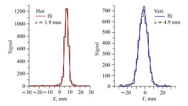
Fig. 3. The X- (left) and Y- (right) coordinate beam profile at the focus F4. The lines are the results of the Gaussian fit
