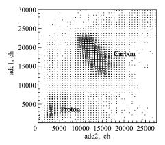
Fig. 5. The signal amplitudes correlation for one of the scintillation detectors of the hodoscope
