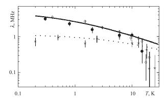
Fig. 4. Temperature dependence of the relaxation rate of the negative muon spin in p-type Ge: closed circles correspond to the Ga concentration  $1.0 \cdot 10^{14} \text{ cm}^{-3}$ ; opened circles, to  $3 \cdot 10^{14} \text{ cm}^{-3}$ ; and crosses, to  $5 \cdot 10^{15} \text{ cm}^{-3}$ . The solid and dotted lines correspond to approximation of the function (2) to the experimental data (see the text)
