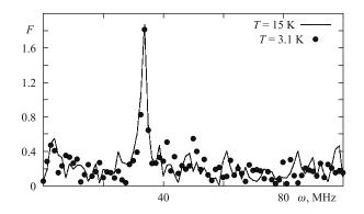
Fig. 3. Fourier analysis of the  $\mu$ SR spectra in the n-type Ge sample at 3.1 K and 15 K
