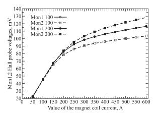
Fig. 6. The dependence of the monitor Hall probes Mon1 and Mon2 readings on the SRM coil current
