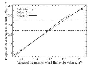
Fig. 8. The dependence of the  $H_Z$  component integral value of the magnetic field induction on the values of the monitor Mon1 Hall probe voltage
