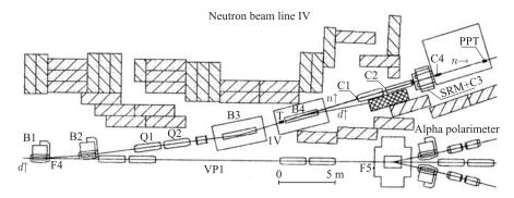
Fig. 1. Polarized neutron beam line IV for the  $\Delta \sigma_L(np)$  experiment. Designations:  $d\uparrow$  — transverse polarized deuteron beam; T — neutron generation target;  $n\uparrow$  — transverse polarized neutron beam; C1–C4 — the neutron beam collimators; SRM — the spin rotation magnet;  $n \rightarrow$  — longitudinally polarized neutron beam; PPT — polarized proton target
