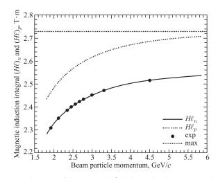
Fig. 2. The calculated values of the magnetic field induction integrals required to rotate the beam neutron  $(H\ell)_n$  and proton  $(H\ell)_p$  spins through the angle of 90° depending on the beam particle momentum. The maximum integral value, which can be obtained by using the prepared spin rotation magnet, is shown by a straight dotted line. The integral values set at the corresponding beam momentum values during the  $\Delta \sigma_L(np)$  data taking runs are shown by the solid circles
