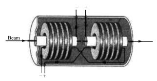
Fig. 8. Typical structure of a ferrite-loaded cavity [17]
