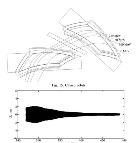
Fig. 16. Axial motion of the particle with initial axial displacement
