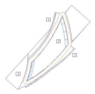
Fig. 4. Spiral sector: 1 — clamps, 2 — pole, 3 — yoke
