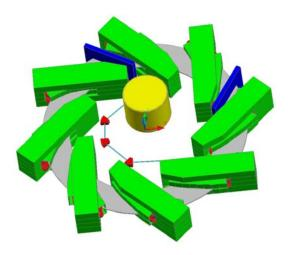
Fig. 1. General layout of the JINR FFAG with the H-injector cyclotron included
