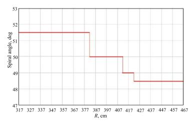
Fig. 5. Sector spiral angle vs. radius. Actually, at the location of the vertices the spiral angle is smoothed in the computer model and in the resulting field distribution in the midplane of the magnet
