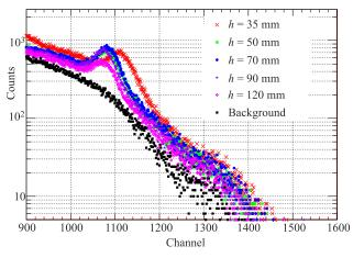
Fig. 10. Pulse height spectra of the  $30 \times 30 \times 130$  mm LYSO crystal irradiated by the <sup>22</sup>Na  $\gamma$  source placed at distances of 35, 50, 70, 90 and 120 mm from the PMT cathode (1786 keV full absorption peaks are around channel 1100)
