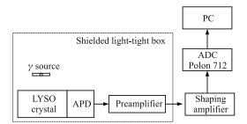
Fig. 3. The block diagram of the setup for measuring the  $10\times10\times10$  mm LYSO crystal energy resolution
