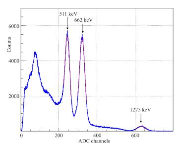
Fig. 13. The  $10\times10\times10$  mm LYSO crystal spectrum due to intrinsic radioactivity and  $^{22}\mathrm{Na}$  and  $^{137}\mathrm{Cs}$  irradiation. Three full absorption peaks are fitted with Gaussians
