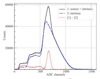
Fig. 6. LYSO spectra due to intrinsic radioactivity and  $^{137}$ Cs irradiation: total spectrum (solid line), spectrum due to intrinsic radioactivity (dashed line), and spectrum due to  $^{137}$ Cs irradiation (dotted line)
