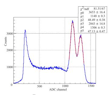
Fig. 7. LYSO spectra due to <sup>60</sup>Co irradiation. Two full absorption peaks corresponding to 1173 and 1333 keV are fitted with the sum of two Gaussians
