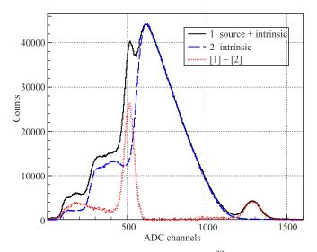
Fig. 5. LYSO spectra due to intrinsic radioactivity and  $^{22}$ Na irradiation: total spectrum (solid line), spectrum due to intrinsic radioactivity (dashed line), and spectrum due to  $^{22}$ Na irradiation (dotted line)
