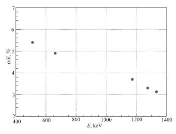
Fig. 14. The  $10 \times 10 \times 10$  mm LYSO crystal energy resolution measured by the S8664-1010 Hamamatsu APD as a function of the photon energy
