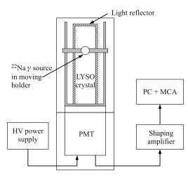
Fig. 2. The block diagram of the setup for measuring the  $30 \times 30 \times 130$  mm LYSO crystal light response uniformity
