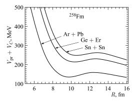
Fig. 7. The nucleus–nucleus potential for the DNS formed from the  $^{258}\mathrm{Fm}$  nucleus during its evolution towards the equilibrium configuration
